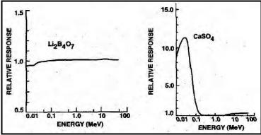
Figure A-1. Typical photon energy response curves for Li<sub>2</sub>B<sub>4</sub>O<sub>7</sub> and CaSO<sub>4</sub> TLD elements (Allen and Schoengold 1995).
