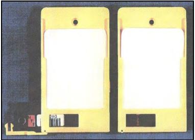
Figure 6-3. REECo security badge holder with Panasonic UD-802 dosimeter.
