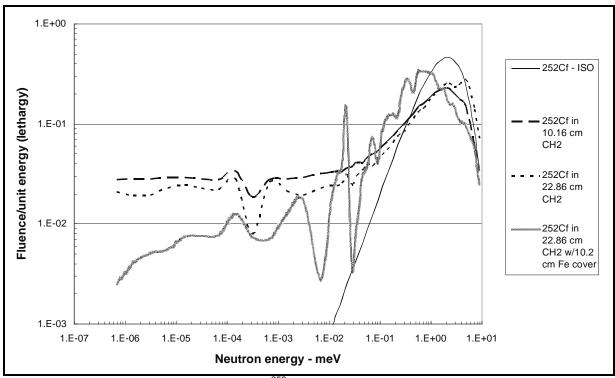
Figure A-8. Lethargy neutron spectra for <sup>252</sup>Cf with various thickness moderators (IAEA 2001).
