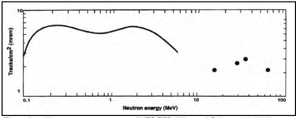
Figure A-5. Neutron energy response of NTS TED (Allen and Schoengold 1995).
