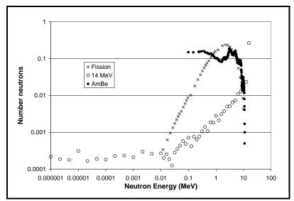
Figure 6-14. Neutron spectra that simulate INL facilities [19].
