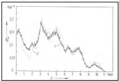
Figure 6-8. Probability density of neutron spectrum from a <sup>241</sup>Am-Be(α,n) source (Kluge and Weiss 1982).
