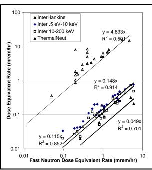
Figure 6-16. MTR neutron field components (ORAUT 2006a).
