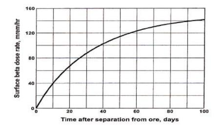
Figure 4. Beta dose rate from yellowcake separated from ore for more than 100 days as a function of distance from the surface. [Reproduced from US NRC 2002b]
