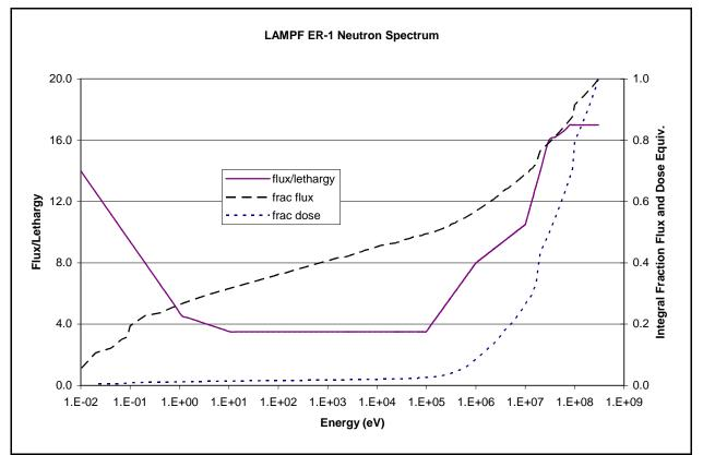
Figure 6-1. Neutron spectrum per unit lethargy and the integral spectrum of flux and dose equivalent for the LAMPF ER-1 spectrum.
