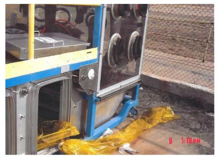
Figure 4. Closeup of Downdraft Table used for W55 Dismantlement Source: [Worker II] 2011
