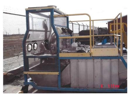
Figure 3. Gloveboxed Downdraft Table, Installed late-1991, for W55 Dismantlement Source: [Worker II] 2011
