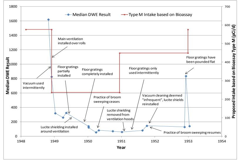
Figure 5. Median Daily Weighted Exposure and Proposed Type M Intakes based on Bioassay Data Plotted versus the Timeline of Significant Changes in Industrial Control
