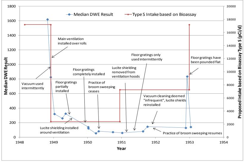
Figure 6. Median Daily Weighted Exposure and Proposed Type M Intakes based on Bioassay Data Plotted versus the Timeline of Significant Changes in Industrial Control
