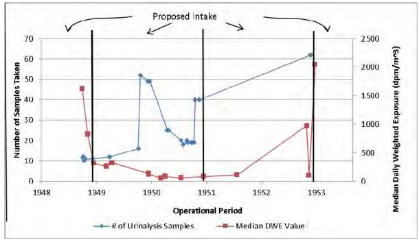
Figure 3. Chronological Plot of the Uranium Urinalysis Sampling versus the Median Daily Weighted Exposure over the same Timeframe
