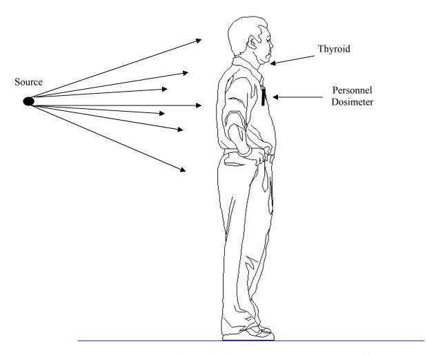
Figure 2.1-3. Worker Receiving Radiation Exposure From Posterior Geometry
