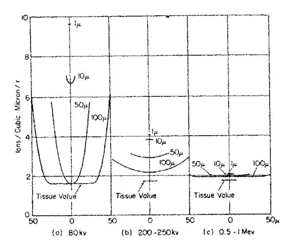
Figure 2.1-2. Ionization in Soft Tissue Inside Bone Cavities for Radiation Generated at 80 kv, 200 to 250 kv, and 0.5 to 1.0 MeV
