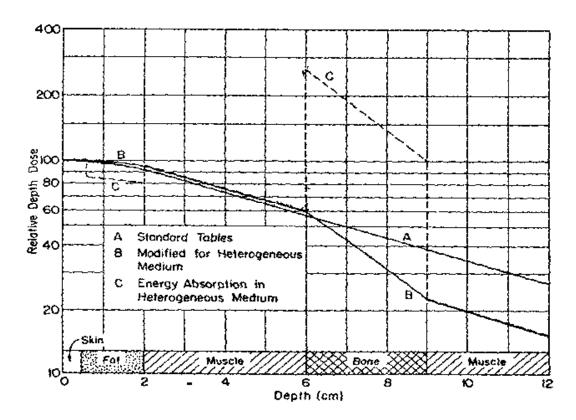
Figure 2.1-1. Relative Depth Dose in a Phantom Consisting of Layers of Skin, Fat, Muscle, and Bone. Field size 100 cm<sup>2</sup>, TSD 50 cm, HVL 1.5 mm Cu. (Spiers 1946)
