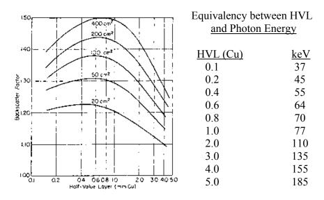
Figure 2.1-6. Variation of the Backscatter Factor with the Quality of the Radiation for a Number of Field Sizes
