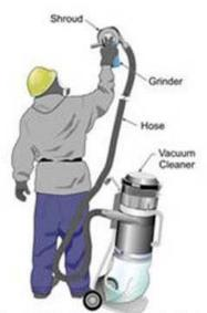
Figure 1. Grinder in use with the control in place.
