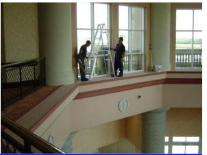
Figure 5. Close up of maintenance workers setting up for an atrium maintenance activity representing a serious fall hazard risk. A design that incorporates guardrails or built-in anchors for use with fall harnesses would substantially reduce this hazard.
