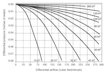
FIGURE 4. Empirical relation between differential airflow, differential pressure, and leakage areas\*
