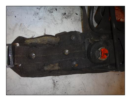
Figure 24: Left side waist strap heat damage
