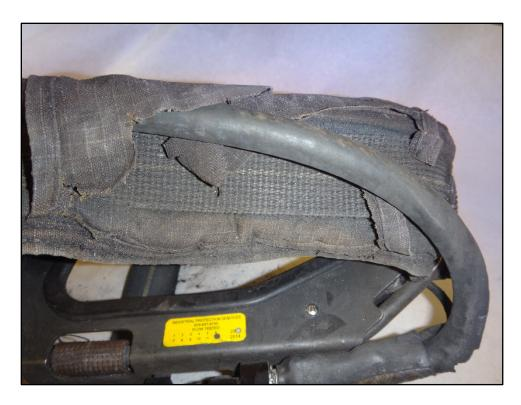
Figure 23: Left side shoulder strap heat damage
