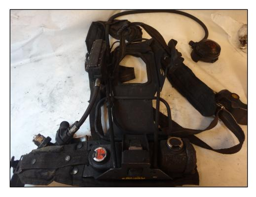
Figure 18: PASS control module heat damage
