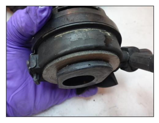
Figure 8: Remnants of label on Mask Mounted Regulator
