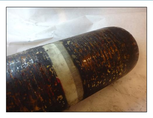
Figure 27: Heat damage to cylinder
