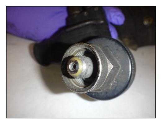
Figure 14: O-ring and threads of cylinder attachment
