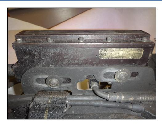
Figure 11: Side of first stage regulator
