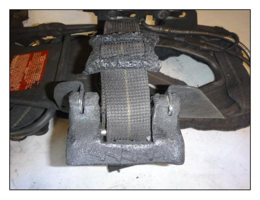
Figure 21: Melted cylinder strap
