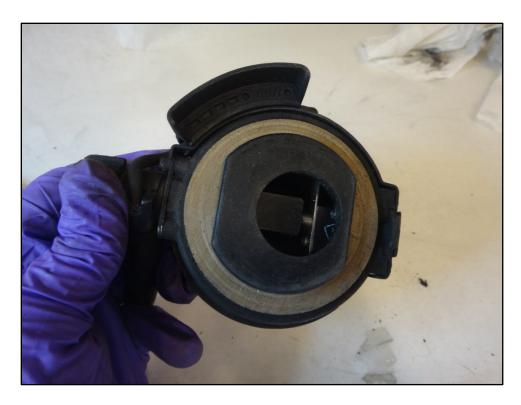
Figure 7: Inside flange of Mask Mounted Regulator
