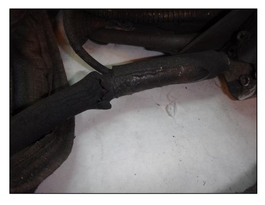
Figure 10: Low pressure hose sheath heat damage
