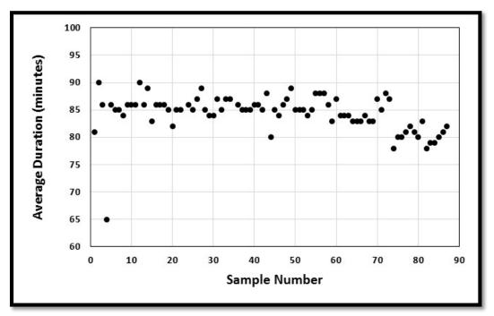
Figure 15. Average Duration of Dräger Oxy K Plus SCSRs
