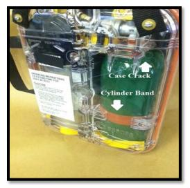
Figure 9. Ocenco EBA 6.5 with Case Crack
