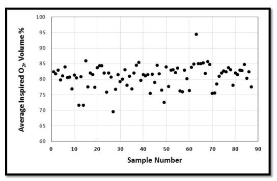
Figure 17. Average Percent Oxygen of Dräger Oxy K Plus SCSRs
