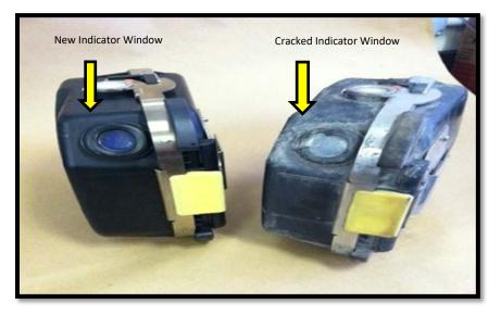
Figure 8. New Moisture Indicator and Cracked Indicator Found After Cleaning at NIOSH
