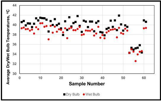
Figure 30. Average Dry/Wet Bulb Temperature of Ocenco M-20 SCSR
