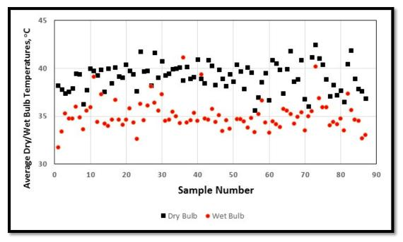
Figure 18. Average Dry Bulb/Wet Bulb Temperature of Dräger Oxy K Plus SCSRs
