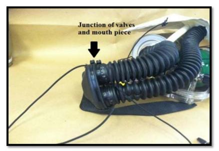
Figure 12. Ocenco EBA 6.5 Junction of Plastic Valves at Mouthpiece
