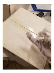
Figure 2: Most amount of dust observed on product cases from Facility Eight.
