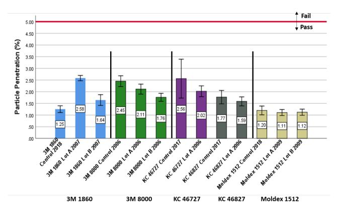
**Figure 7:** Control and stockpiled respirator particle filtration performance data. N95 FFRs must have a particle penetration of less than 5.0%. Error bars represent the 99% confidence interval and estimate the population parameters. This confidence interval suggests that 99% of any repeated samples tested and evaluated from this lot will have a mean between the upper and lower bounds.
