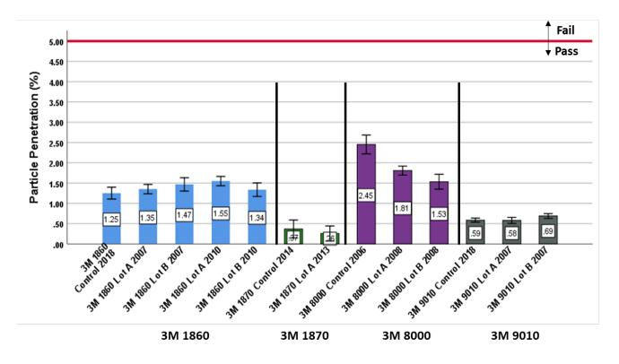
**Figure 9:** Control and stockpiled respirator particle filtration performance data for the 3M 1860, 3M 1870, 3M 8000, and 3M 9010 models. N95 FFRs must have a particle penetration of less than 5.0%. Error bars represent the 99% confidence interval and estimate the population parameters. This confidence interval suggests that 99% of any repeated samples tested and evaluated from this lot will have a mean between the upper and lower bounds.
