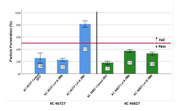
**Figure 12:** Control and stockpiled respirator particle filtration performance data for the KC 46727 and KC 46827 models. N95 FFRs must have a particle penetration of less than 5.0%. Error bars represent the 99% confidence interval and estimate the population parameters. This confidence interval suggests that 99% of any repeated samples tested and evaluated from this lot will have a mean between the upper and lower bounds.
