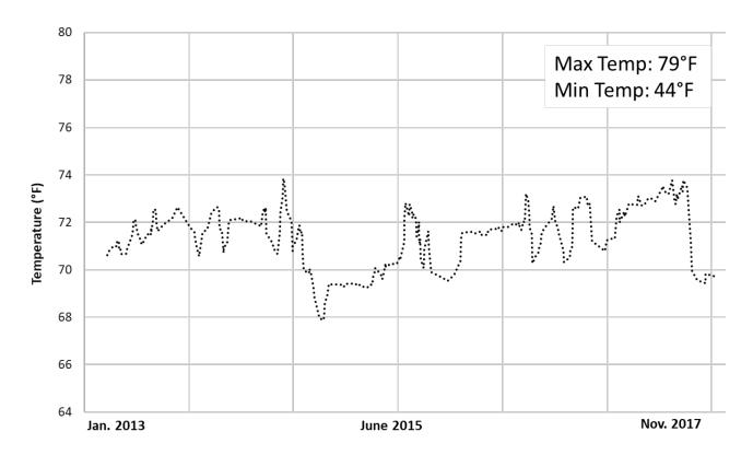
**Figure 4:** Temperatures from January 2013 – November 2017 taken at five locations within Facility Six. Data is plotted as a 5-point moving average for visualization purposes. Maximum and minimum temperatures reported are noted for each data logger.
