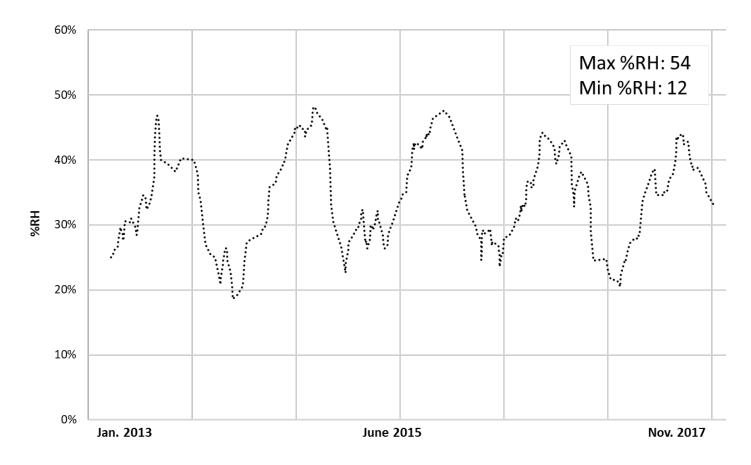
**Figure 3:** Percent Relative Humidity (% RH) from January 2013 – November 2017 taken at one location within Facility Six. Data is plotted as a 5-point moving average for visualization purposes. Maximum and minimum temperatures reported are noted for each data logger.
