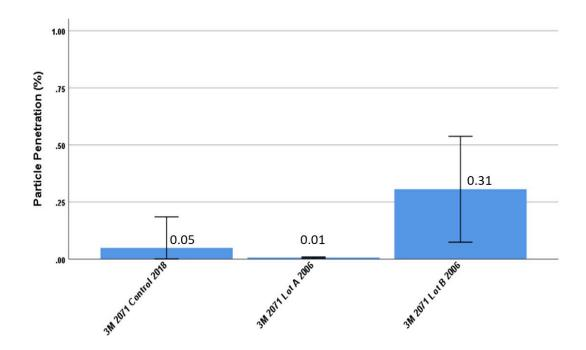
**Figure 11:** Control and stockpiled respirator particle filtration performance data for the 3M 2071 model. P95 filters must have a liquid particle penetration of less than 5.0%. Error bars represent the 99% confidence interval and estimate the population parameters. This confidence interval suggests that 99% of any repeated samples tested and evaluated from this lot will have a mean between the upper and lower bounds.
