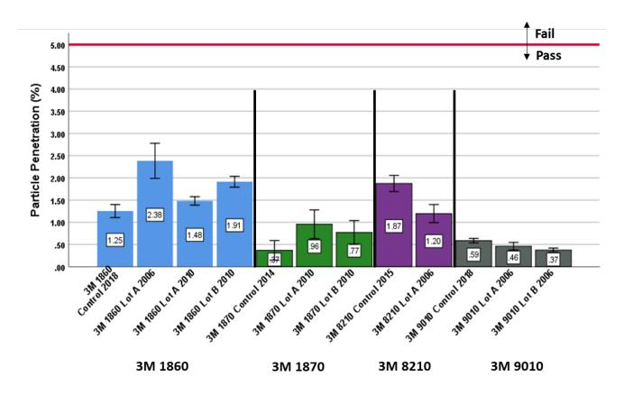
**Figure 10:** Control and stockpiled respirator particle filtration performance data for the 3M 1860, 3M 1870, 3M 8210, and 3M 9010 models. N95 FFRs must have a particle penetration of less than 5.0%. Error bars represent the 99% confidence interval and estimate the population parameters. This confidence interval suggests that 99% of any repeated samples tested and evaluated from this lot will have a mean between the upper and lower bounds.
