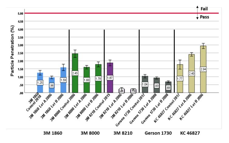
**Figure 6:** Control and stockpiled respirator particle filtration performance data. N95 FFRs must have a particle penetration of less than 5.0%. Error bars represent the 99% confidence interval and estimate the population parameters. This confidence interval suggests that 99% of any repeated samples tested and evaluated from this lot will have a mean between the upper and lower bounds.
