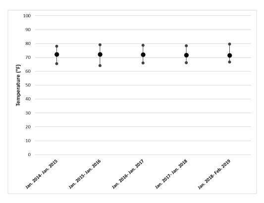
**Figure 4:** Temperatures from January 2014 – February 2019 for 96 temperature probes stored at Facility Ten. Data is plotted as minimum, maximum, and average temperatures.
