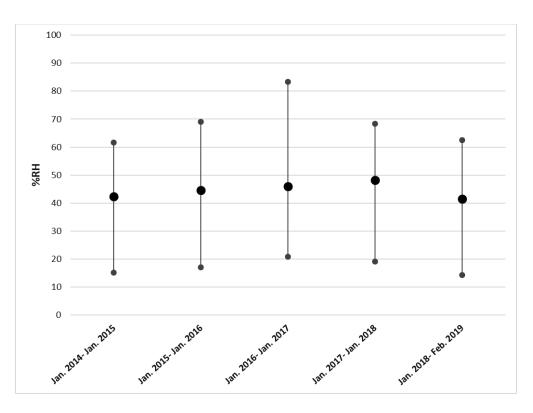
**Figure 3:** Percent Relative Humidity (% RH) from January 2014 – February 2019 for one %RH probe stored at Facility Ten. Data is plotted as minimum, maximum, and average %RH.
