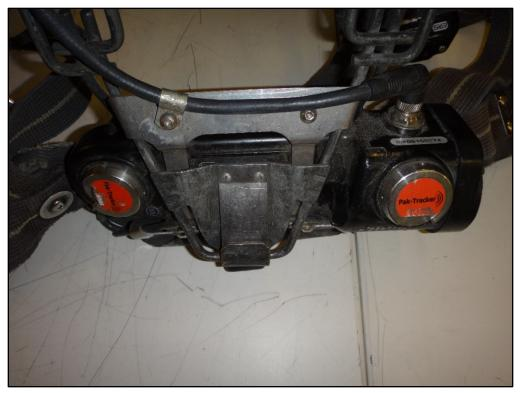
Figure 14: PASS control module
