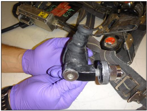
Figure 9: Cylinder attachment overview and relief valve
