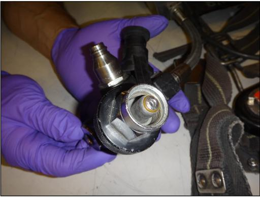
Figure 11: Quick fill port on cylinder attachment and overview of threads
