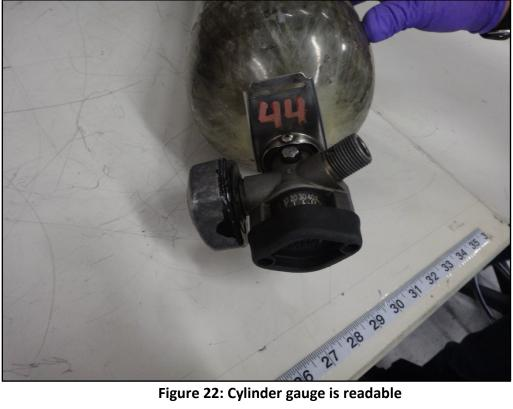
Figure 22: Cylinder gauge is readable
