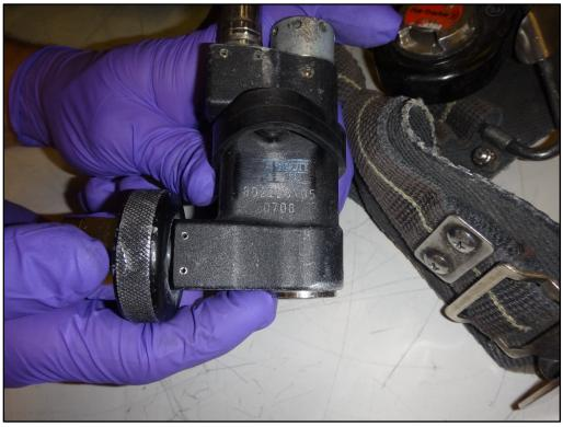
Figure 10: Cylinder attachment identifying markings
