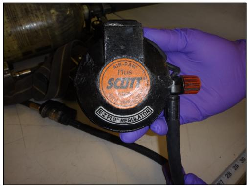
Figure 3: Mask mounted regulator
