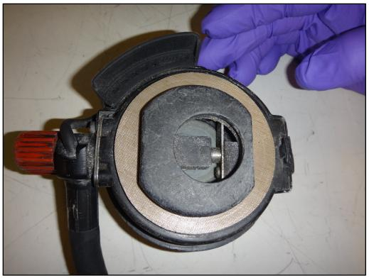
Figure 4: Inside flange, Mask mounted regulator
