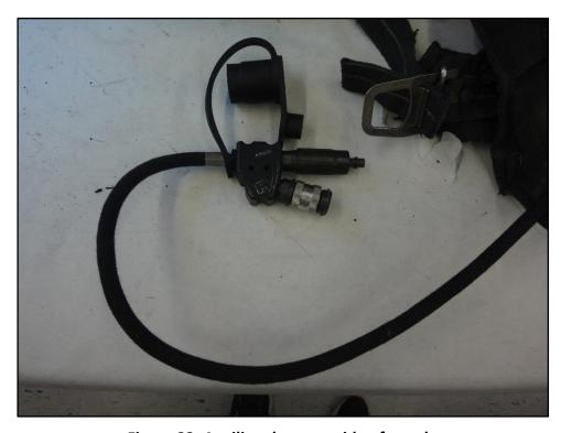
Figure 23: Auxiliary hose outside of pouch.
