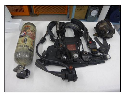
Figure 3: SCBA unit, facepiece, and cylinder out of bag.
