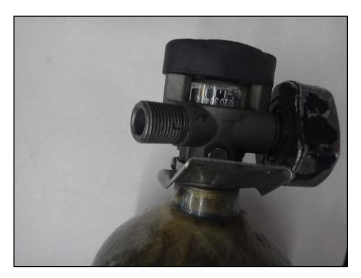
Figure 27: Cylinder gauge is legible, view of threads.
