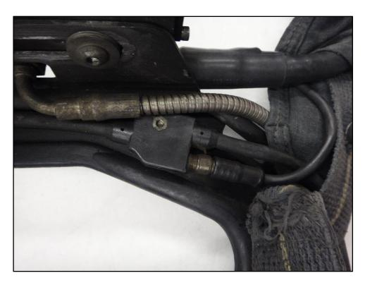
Figure 10: Low pressure regulator hose and HUD connection.
