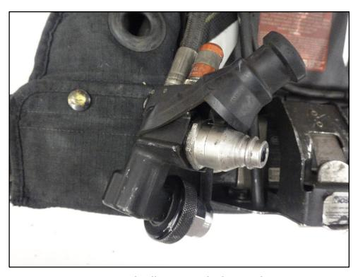
Figure 15: Quick-Fill port on cylinder attachment.
