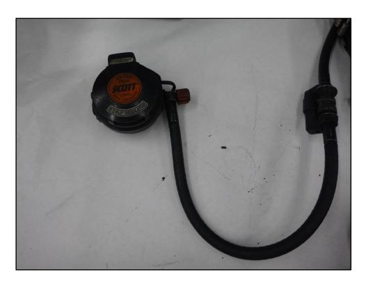
Figure 9: MMR, low pressure with Quick Disconnect.
