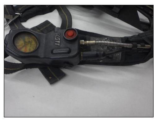
Figure 16: High pressure line to PASS console
