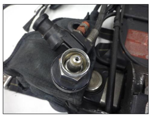
Figure 14: Cylinder attachment threads.
