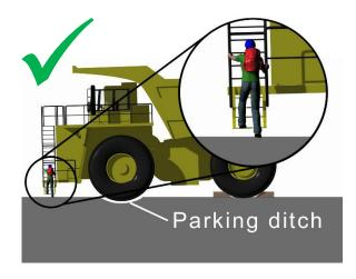
**Solution:** Create a parking ditch in a designated parking area. Resting the front wheels in the ditch lowers the height of the front of the equipment, and thereby decreases the height of the first step. This serves also to further immobilize the equipment.
