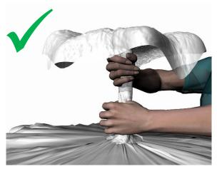
**Solution:** Encourage workers to use the "flowering method" to close bulk bags, where the bag material is just gathered at the top and the worker uses a pneumatic cable tie gun with cable ties to seal the bulk bag. This method lowers injury risk when closing and sealing bulk bags.
