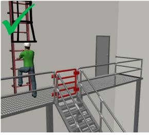
**Solution:** Ensure the tops of stairways and ladders are offset and equipped with self-closing gates that open inward to reduce the potential for workers to fall.
