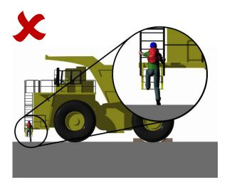
**Problem:** When parking heavy mobile equipment on a level surface, the distance from the ground to the first step of the access ladder may be large. This makes ingress more strenuous and can increase injury risks when stepping off of the equipment.
