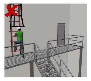
**Problem:** Shared landings create unique hazards at facilities because a fall from a ladder can also cause a fall down the stairs.
