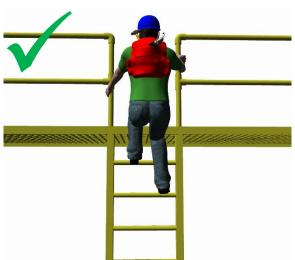
**Solution:** Supply workers with a backpack to hold lightweight tools while climbing a ladder to ensure safe transport of tools while maintaining three points of contact. If the tools or supplies are heavy, they should not be carried (even in a backpack) up or down a ladder.
