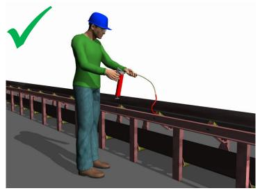
**Solution:** Add an access line so the worker can stand upright while greasing.
