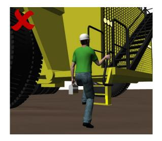
**Problem:** A driver climbing a ladder or stairway when boarding mobile machinery and carrying a lunch box is not able to safely maintain three points of contact.
