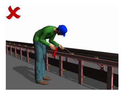
**Problem:** Without an access line, the worker has to bend to access the grease fitting and for the remaining time spent greasing.
