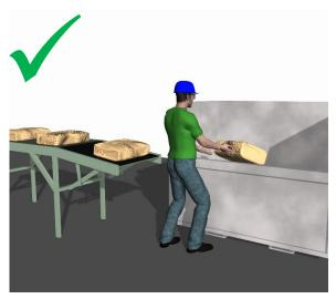
**Solution:** Provide a redesigned dumpster with a lowered front edge to facilitate lifting in the power zone between the waist and shoulder. This reduces the stress associated with working at or above shoulder height.
