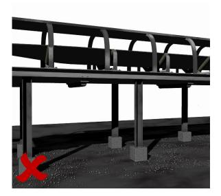
**Problem:** Spillage from conveyers and belts can encroach onto neighboring walkways or paths of travel and lead to a slip or fall. When wet, some materials can be especially dangerous in that these materials may increase the likelihood of slips.
