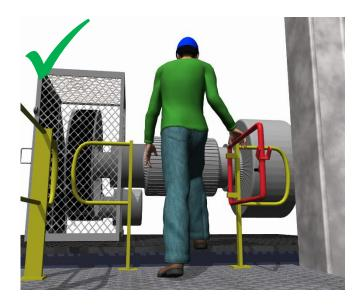
**Solution:** Improve equipment access by replacing sections of guarding with secured gates. This prevents workers from unintentional contact with equipment while allowing them access when needed.
