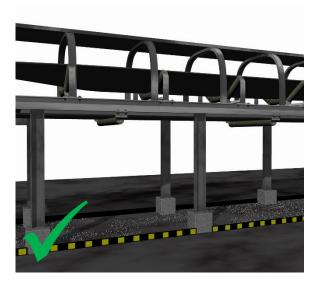
**Solution:** Add a barrier adjacent to the walkways to prevent spillage from entering walkways and causing slips. For example, a toe plate added along a conveyor and adjacent to the walkway could stop conveyor spillage from entering the walkway. If the toe plate is brightly colored and clearly marked, it helps prevent tripping when working close to or under the conveyor.
