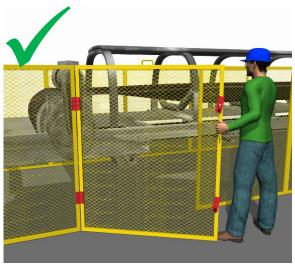
**Solution:** Design area guards so they are easily handled by a single worker. Guards may be mounted on door hinges that allow them to open easily when access is needed.
