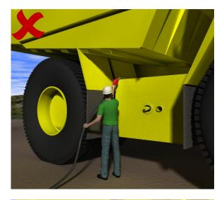
**Problem:** Mobile equipment fueling stations commonly have nozzles and fueling points located at or above shoulder height. Similarly, the gas tank cap may also be located above shoulder height. Reaching above shoulder height can increase the risk of injury to the arms and shoulders.
