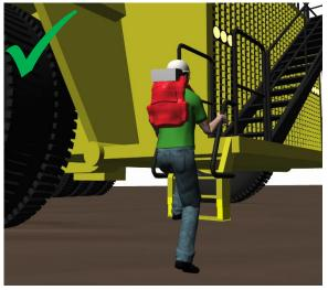
**Solution:** Supply drivers with a backpack to transport their personal items safely while maintaining three points of contact.
