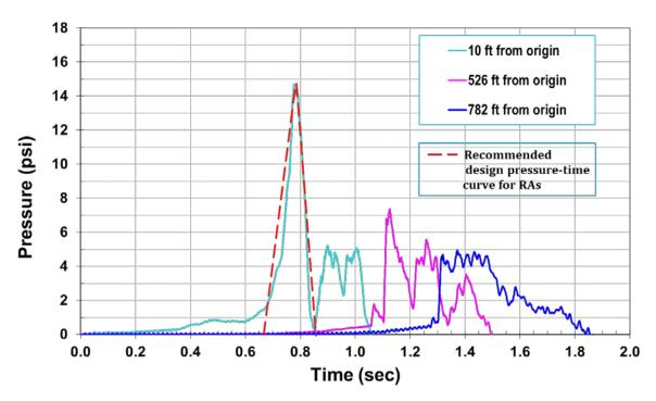
Figure 4. Pressure-time curve showing pressure decay with distance and shock wave development from LLEM test #485 with 60-ft gas zone.
