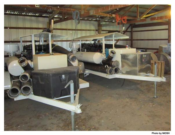
Figure A6. Portable, diesel-powered blowers for borehole air supply systems.
