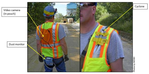
Figure 3. Setup of sampling devices for personal sampling.
