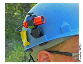
Figure 4. Placement of the video camera lens on the helmet.
