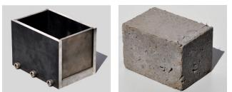
Figure 2. Partial beam box mold and test specimen.
