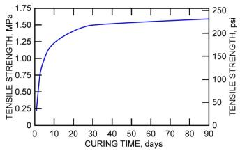
Figure 4. Typical shotcrete adhesion test results.
