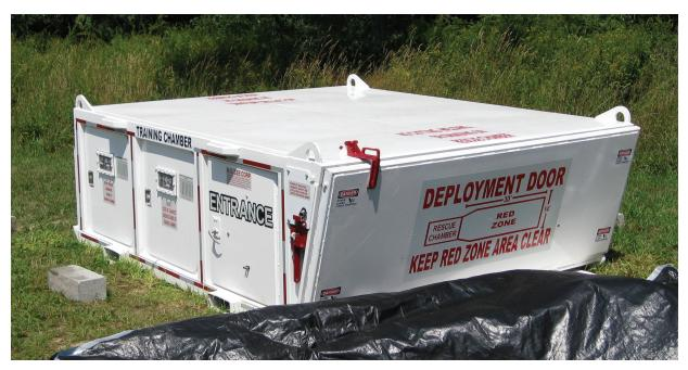
Figure 2. Training model of an inflatable refuge chamber.
