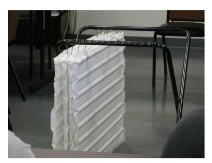
**Figure 3.** Mock-up of scrubber curtains and the stand used to hold them.
