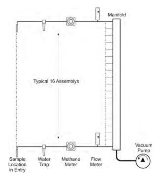
Figure 10. Methane sampling system.
