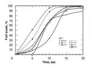
Figure 70. Response times for person-wearable monitors.
