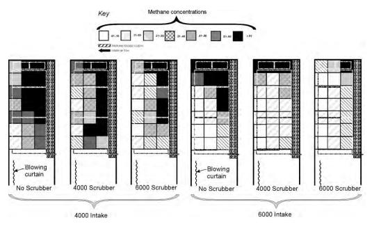
Figure 43. Methane concentrations above mining machine.
