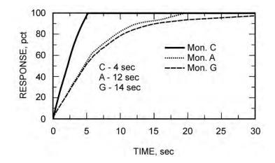
Figure 59. Response times measured in test box (dust cap off).
