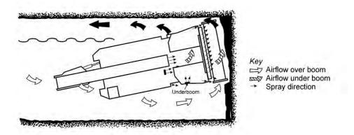
Figure 4. Spray fan system used to move air across the face.
