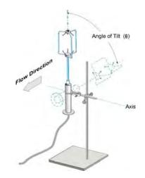
Figure 83. Evaluating effect of tilt angle on airflow readings.
