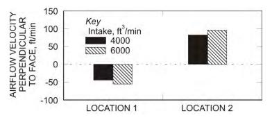
Figure 47. Airflow with no water sprays operating at locations 1 and 2 shown in Figure 45.
