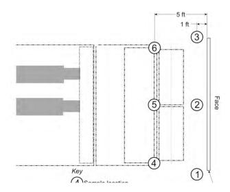
Figure 21, Methane sampling locations for curtain/tubing tests.
