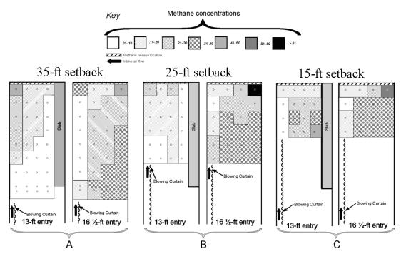
Figure 27. Methane profiles with 10,000 ft3/min curtain flow for 13- and 16<sup>1</sup>/<sub>2</sub>-ft entries at a 35-ft curtain setback (A), 25-ft curtain setback (B), and 15-ft curtain setback (C).
