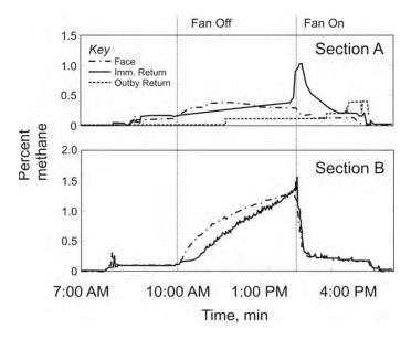
Figure 75. Accumulation of gas at two faces in one mine.
