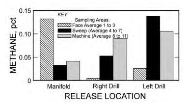
Figure 89. Effects of release location on concentration.
