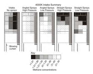
Figure 50. Methane distribution, 4,000 ft3/min intake flow.
