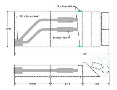
Figure 6. Model mining machine showing scrubber.
