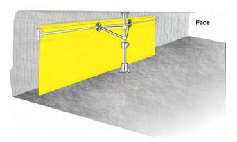
Figure 2. Extensible curtain suspended from a rail and rollers.
