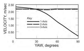
Figure 82. Effect of yaw angle on anemometer readings.
