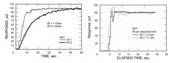
Figure 61. Response times with dust caps on (left plot) and off (right plot).
