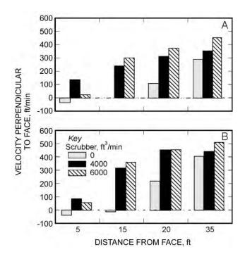
Figure 29. Airflow toward the face for 4,000-ft3/min intake (A) and 6,000-ft3/min intake (B).
