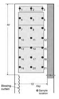
Figure 42. Methane sampling locations above mining machine (scrubber tests).
