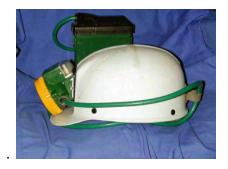
Figure 71. Cap lamp-mounted methane monitor.
