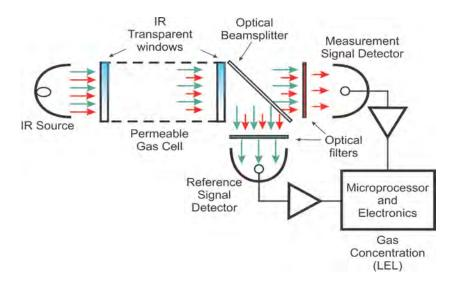
Figure 54. Components of infrared sensor.
