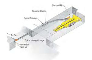
Figure 12. Spiral reinforced tubing attached to mining machine.
