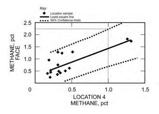
Figure 67. Comparison of face methane concentrations versus concentrations at location 4 (return air side, 5.5 ft from the face).
