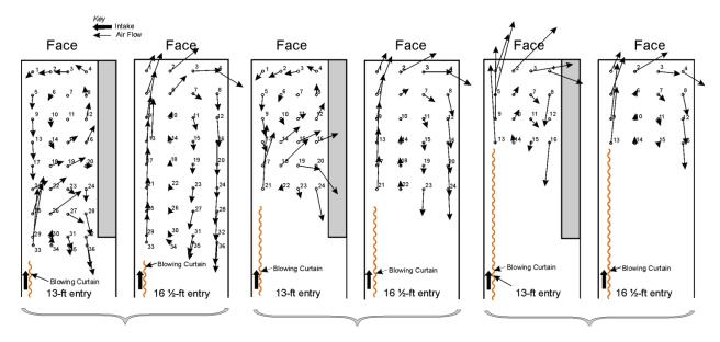
Figure 25. Flow profiles with 10,000 ft3/min curtain flow for 13- and 16½-ft entries at a 35-ft curtain setback (A), 25-ft curtain setback (B), and 15-ft curtain setback (C).
