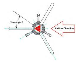
Figure 81. Measuring a yaw angle.
