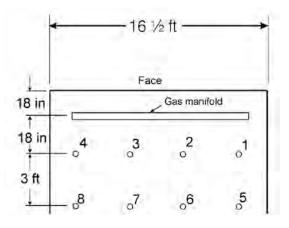
Figure 19. Face sampling locations for jet fan tests.
