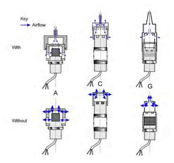
Figure 58. Sensor heads (A, C, and G) with and without the calibration cups attached.
