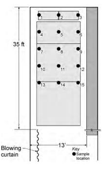
Figure 49. Methane sampling locations above mining machine (water spray tests).
