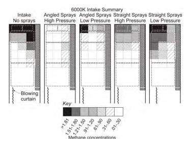
Figure 51. Methane distribution, 6,000 ft3/min intake flow.
