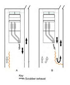
Figure 38. Airflows with blowing (A) and exhausting (B) conditions at a 35-ft setback distance.
