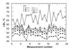
Figure 69. Daily readings for person-wearable monitors.
