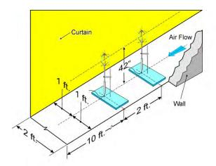
Figure 78. Airflow sampling locations behind the curtain.
