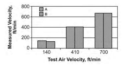
Figure 79. Velocity readings for three flows measured with two, 3-axis anemometers.
