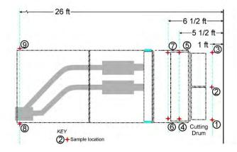
mining machine. In addition, there were three sampling locations 1 ft from the face (Figure 65).
