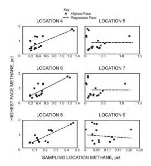
Figure 66. Comparison of measurements on mining machine. Locations given in Figure 65.
