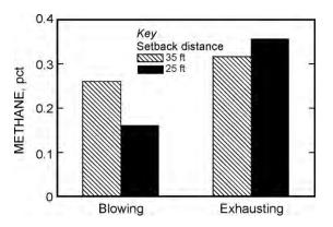
Figure 40. Effect of setback distance on methane concentration with scrubber operating.
