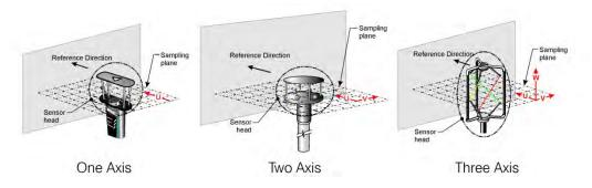
Figure 76. Ultrasonic sensor heads with flow components.
