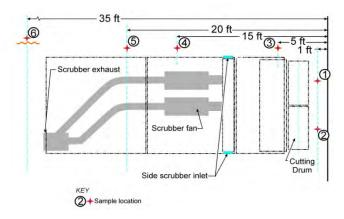
Figure 28. Airflow measurement locations with mining machine at the face.
