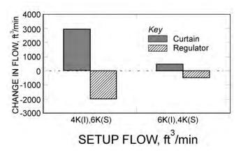
Figure 35. Changes in intake flow measured at curtain and regulator due to operation of the scrubber.
