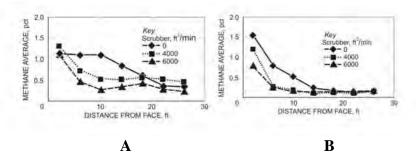
Figure 44. Dilution of methane at intake flows of 4,000 ft3/min (A) and 6,000 ft3/min (B).
