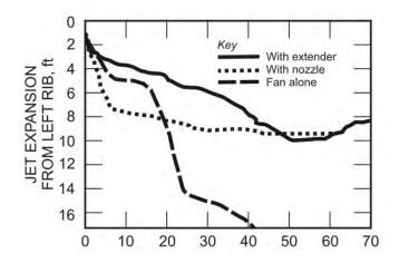
Figure 16. Airflow profiles for three jet fan configurations.
