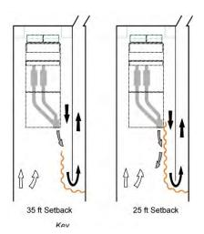
Figure 41. Airflow patterns using a scrubber with exhaust ventilation (35- and 25-ft curtain setbacks).
