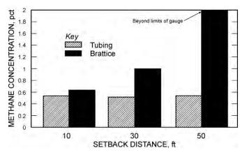
Figure 22. Average face methane concentration with tubing or curtain.
