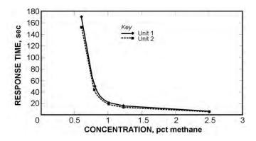
Figure 72. Instrument alarm times (calibration gas 0.6% to 2.5%).
