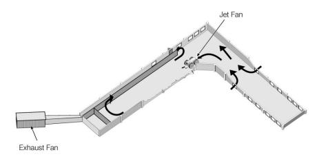
Figure 14. Jet fan test area in ventilation test gallery.
