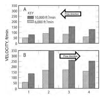
Figure 26. Face velocities at a 25-ft setback for the 13-ft wide entry (A) and the 16<sup>1</sup>/<sub>2</sub>-ft wide entry (B).
