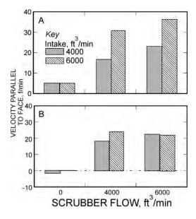
Figure 30. Airflow parallel to face at location 1 (A) and location 2 (B).
