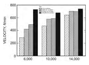
Figure 33. Effect of scrubber flow on intake air quantity.
