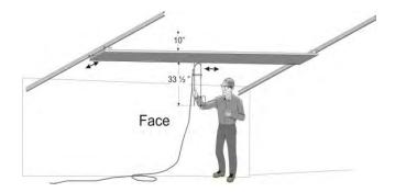
Figure 11. Overhead support system for anemometers.
