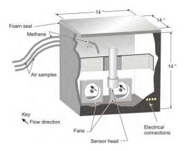
Figure 55. Test box used for response time measurements.
