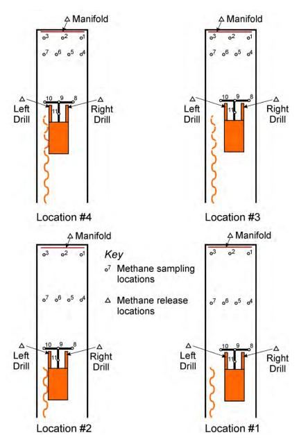
Figure 88. Methane sampling locations for roof bolter tests.
