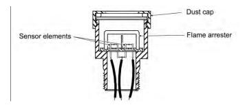
Figure 53. Sampling head with catalytic heat of combustion sensor.
