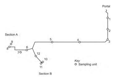
Figure 74. Methane sampling locations in one mine.
