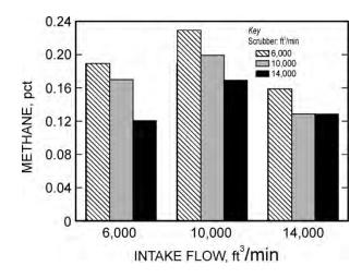
Figure 32. Effects of intake and scrubber flow on methane concentrations.
