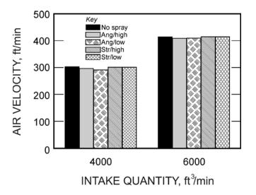
Figure 46. Airflow at mouth of blowing curtain with angled versus straight sprays and high versus low pressure.
