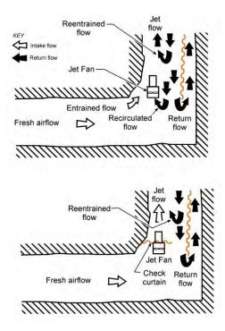
Figure 18. Use of curtain to reduce recirculation.
