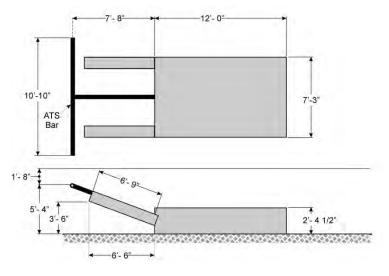
Figure 8. Model roof bolting machine.
