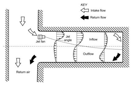
Figure 13. Expansion of jet in mine opening.
