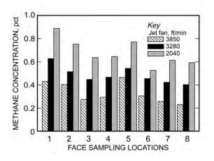
Figure 20. Effect of jet fan velocity on face concentrations.
