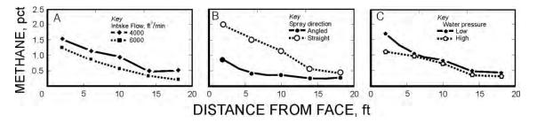
Figure 52. Effect of intake flow (A), nozzle direction (B), and water pressure (C) on concentration versus distance from face.
