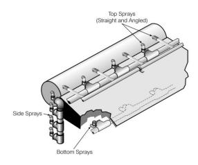
Figure 7. Water sprays on model mining machine.
