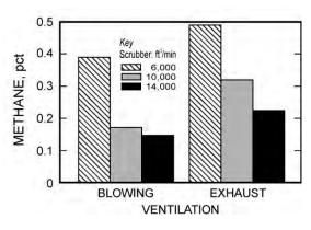
Figure 39. Effects of scrubber use with blowing and exhausting face ventilation.
