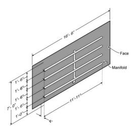
Figure 9. Gas manifold at the test gallery face.
