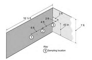
Figure 85. Face airflow sampling locations.
