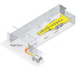
Figure 17. Rigid ducting on jet fan used to reduce recirculation.
