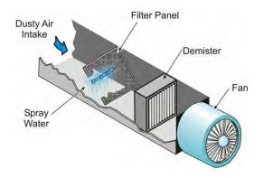
Figure 3. Flooded bed scrubber design.
