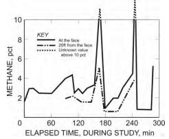
Figure 1. Methane concentrations measured in face area [USBM 1958].
