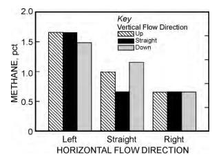
Figure 37. Effect of scrubber exhaust direction on face concentration.
