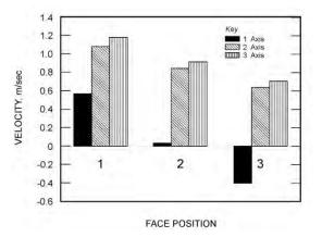
Figure 86. Anemometer readings at face sampling locations.
