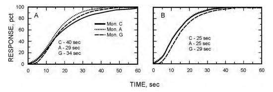
Figure 57. Response times measured with calibration cup (A) and test box (B).
