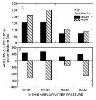
Figure 48. Airflow at curtain (A) and off-curtain (B) side of face.
