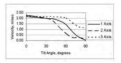
Figure 84. Effect of tilt angle on airflow readings.
