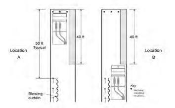
Figure 23. Mining machine locations for measuring face airflow.
