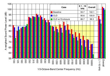
Figure 4.—Sound power level data show an improvement over the CLD configuration of up to 4 dB in the 1- to 10-kHz frequency range with a damped steel-paneled enclosure.
