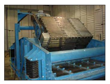
Figure 3.—Completed mechanism enclosure.
