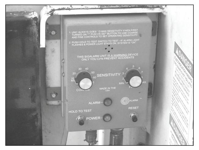
Figure 1.—SIGALARM Model 210 control unit.
