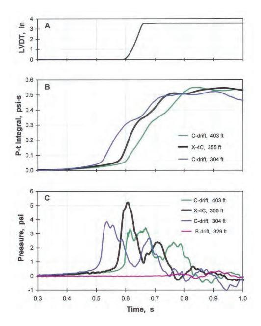
Figure 33.—(A) LVDT displacement, (B) pressure-time integrals, and (C) pressures versus time at dry-stacked hollow-core concrete block stopping in X-4 during LLEM test #428.
