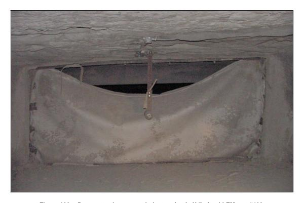
Figure 106.—Damage to the woven cloth stopping in X-7 after LLEM test #462.
