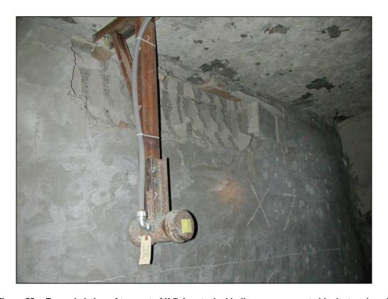
Figure 55.—Expanded view of top part of X-7 dry-stacked hollow-core concrete block stopping after explosion test #433, showing damaged blocks.
