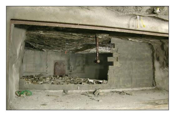
Figure 91.—Damage to the X-4 dry-stacked hollow-core concrete block stopping between B- and C-drifts after LLEM test #497.
