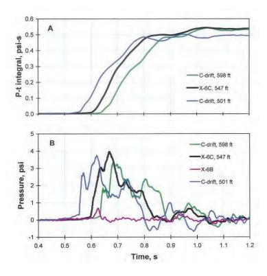
Figure 99.—(A) Pressure-time integrals and (B) pressures at the X-6 woven cloth stopping during LLEM test #460.
