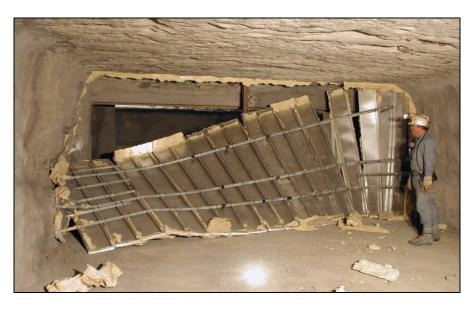
Figure 66.—Debris from steel panel stopping in X-7 after LLEM test #458, viewed from B-drift.
