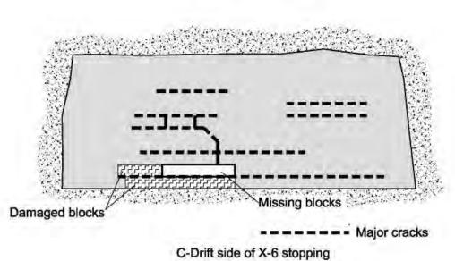
Figure 44.—Expanded cross-sectional views of the blocks remaining in X-6 after test #430.
