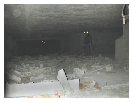
Figure 34.—Debris from dry-stacked hollow-core concrete block stopping in X-4 after LLEM test #428, viewed from C-drift.
