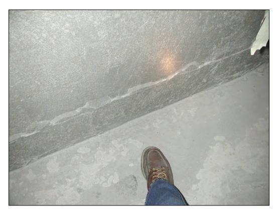
Figure 70.—Displacement of the second block course at the X-4 dry-stacked solid-concrete-block stopping after LLEM test #459, viewed from C-drift.
