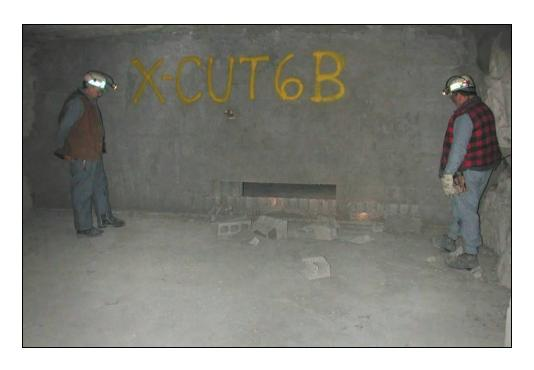
Figure 45.—Crosscut 6 dry-stacked hollow-core concrete block stopping viewed from B-drift side after LLEM test #430, showing blocks dislodged by explosion.
