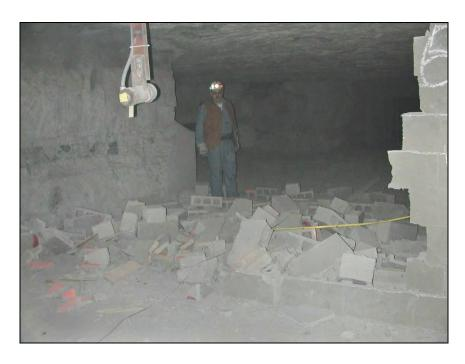
Figure 50.—Debris from X-6 dry-stacked hollow-core concrete block stopping after LLEM test #433, viewed from C-drift.
