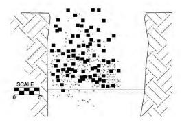
Figure 52.—Expanded map of debris from the X-6 dry-stacked hollow-core concrete block stopping after LLEM test #433. Black squares represent whole or partial blocks, and smaller markings represent pieces of blocks.
