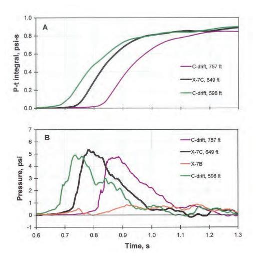
Figure 104.—(A) Pressure-time integrals and (B) pressures at the X-7 woven cloth stopping during LLEM test #462.
