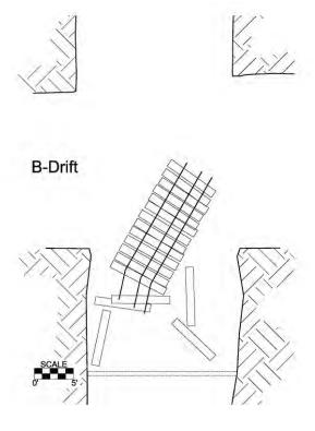
Figure 64.—Map of debris from the X-6 steel panel stopping after LLEM test #458.
