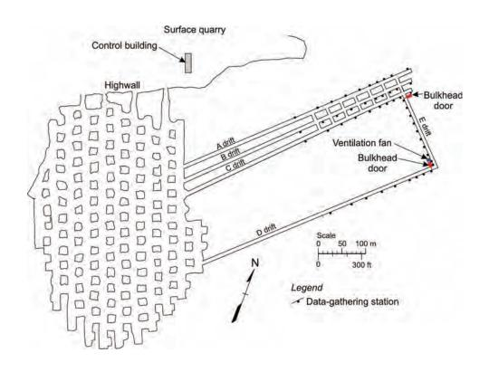
Figure 1.—Plan view of the Lake Lynn Experimental Mine.
