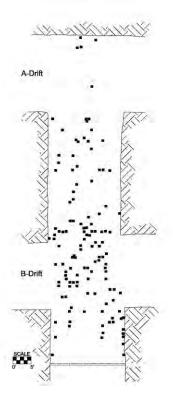
Figure 74.—Map of debris from the X-4 dry-stacked solid-concrete-block stopping after LLEM test #462. Black squares represent whole or partial blocks (smaller block pieces are not shown).
