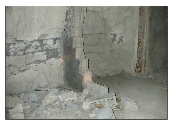
Figure 39.—Remnants of the dry-stacked hollow-core concrete block stopping in X-5 after LLEM test #428. The block shearing indicates roof-to-floor arching action.
