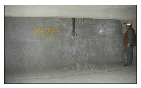
Figure 54.—Condition of X-7 dry-stacked hollow-core concrete block stopping after explosion test #433, viewed from C-drift side.
