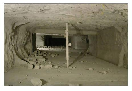
Figure 84.—Debris from 6-in (15-cm) thick, wet-laid solid block stopping in X-7 after LLEM test #519, viewed from A-drift.
