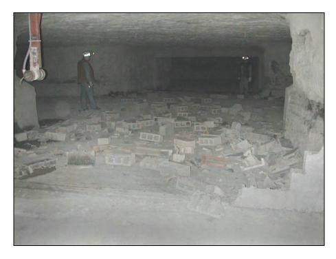
Figure 37.—Debris from X-5 dry-stacked hollow-core concrete block stopping after LLEM test #428, viewed from C-drift.
