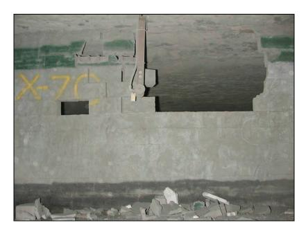
Figure 60.—Crosscut 7 dry-stacked hollow-core concrete block stopping viewed from C-drift after LLEM test #434.
