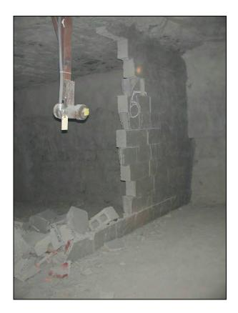
Figure 51.—Part of the inby side of X-6 dry-stacked hollow-core concrete block stopping remaining after LLEM test #433, viewed from C-drift.
