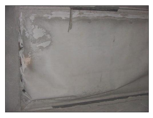
Figure 101.—Tears in the woven cloth on the outby rib of X-6 stopping after LLEM test #460, viewed from C-drift.
