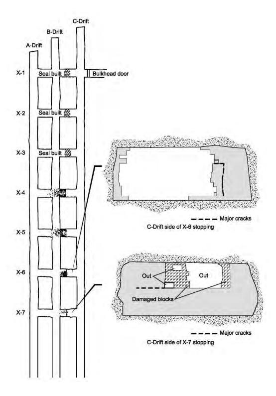
Figure 57.—Effects of explosion test #434 on the dry-stacked hollow-core concrete block stoppings, with expanded cross-sectional views of the blocks remaining in X-6 and X-7.
