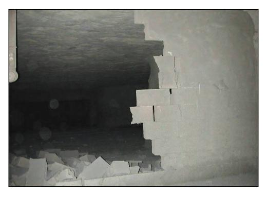
Figure 58.—Additional blocks partially dislodged from the right side of X-6 dry-stacked hollow-core concrete block stopping after test #434, viewed from C-drift.
