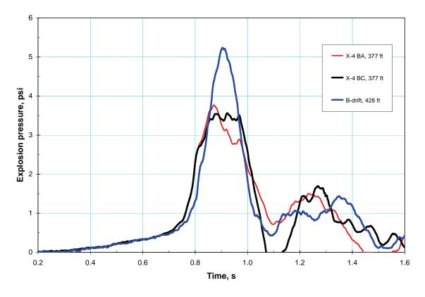
Figure 96.—Total explosion pressures versus time at the dry-stacked hollow-core concrete block stoppings in X-4 and in B-drift during LLEM test #497.
