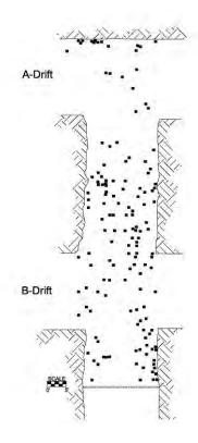
Figure 79.—Debris map for the X-5 dry-stacked solid-concrete-block stopping after LLEM test #463. Black squares represent whole or partial blocks (smaller block pieces are not shown).
