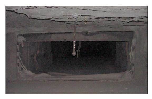
Figure 105.—Damage to the woven cloth stopping in X-6 after LLEM test #462.
