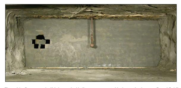
Figure 94.—Damage to the X-3 dry-stacked hollow-core concrete block stopping between B- and C-drifts after LLEM test #497.
