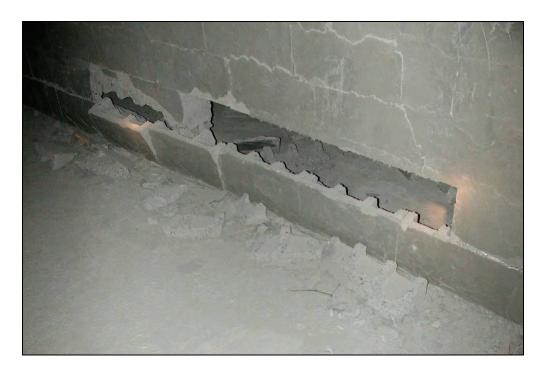
Figure 47.—Closeup of C-drift side X-6 dry-stacked hollow-core concrete block stopping after test #430, showing missing and damaged blocks.
