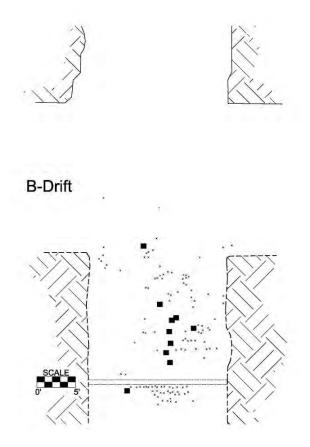
Figure 61.—Map of debris from the X-7 dry-stacked hollow-core concrete block stopping after LLEM test #434. Black squares represent whole or partial blocks, and smaller markings represent pieces of blocks.
