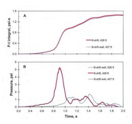
Figure 88.—(A) Pressure-time integrals and (B) pressures versus time at the dry-stacked hollow-core concrete block stopping across B-drift during LLEM test #497.
