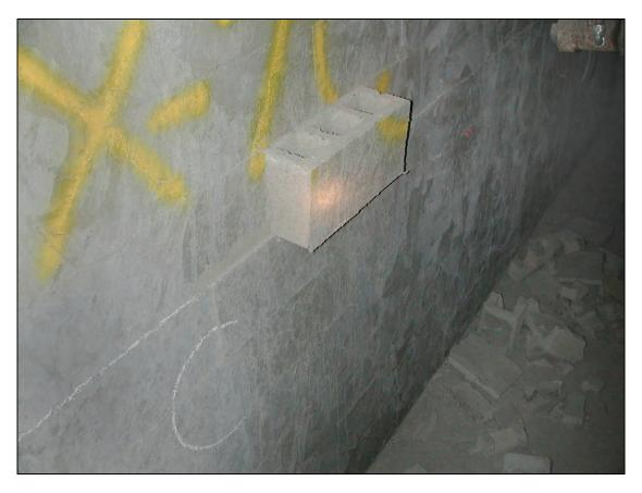
Figure 56.—Expanded view of hollow-core concrete block that is almost dislodged from X-7 dry-stacked stopping after explosion test #433.
