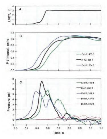
Figure 71.—(A) LVDT displacement, (B) pressure-time integrals, and (C) pressures versus time at the dry-stacked solid-concrete-block stopping in X-4 during LLEM test #462.
