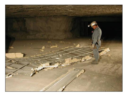
Figure 63.—Debris from steel panel stopping in X-6 after LLEM test #458, viewed from C-drift.
