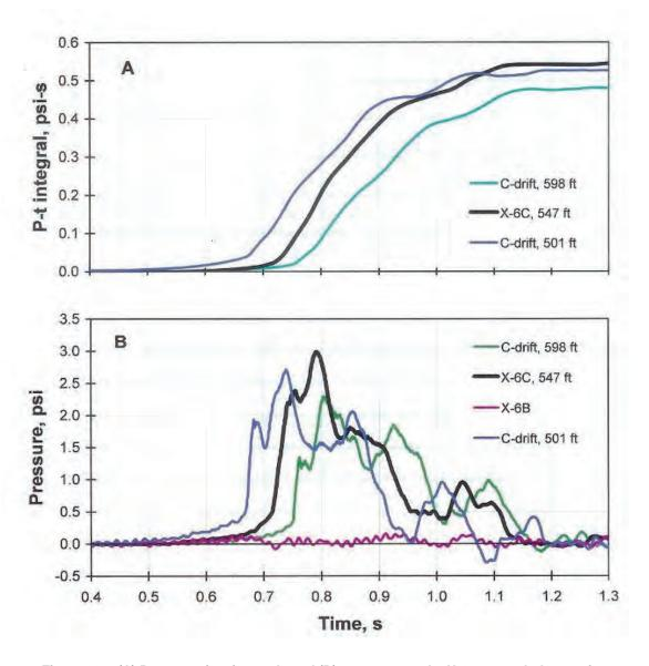
Figure 97.—(A) Pressure-time integrals and (B) pressures at the X-6 woven cloth stopping during LLEM test #459.
