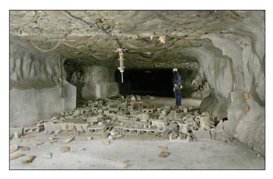
Figure 89.—Debris from the dry-stacked hollow-core concrete block stopping across B-drift after LLEM test #497.
