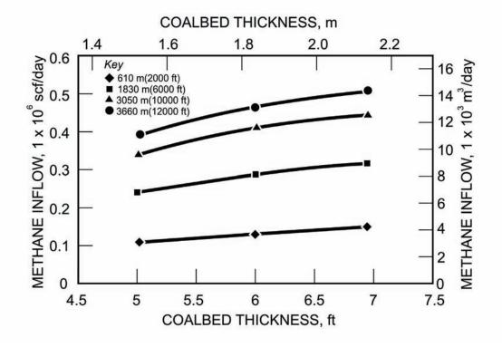
Figure 8.—Effect of coalbed thickness on predicted methane inflow rates into entries of various lengths using reservoir simulation models.
