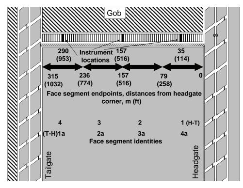
Figure 14.—Pittsburgh Coalbed longwall face emission study site with instrument locations and face segment identities (not to scale).
