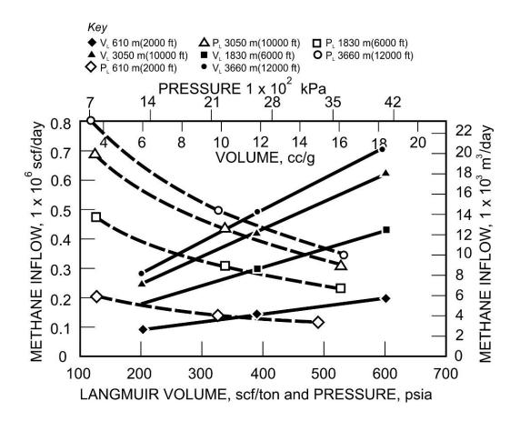
Figure 6.—Effects of Langmuir pressure ( $P_L$ ) and Langmuir volume ( $V_L$ ) on simulated methane inflow rates.
