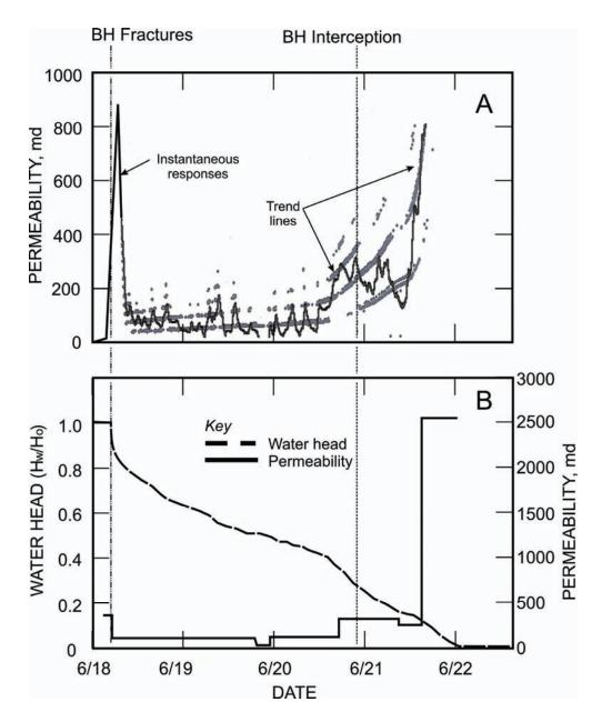
Figure 32.—A: BH–1 instantaneous change in the permeabilities of monitored horizons during mining; B: BH–1 average permeabilities at certain intervals of water head drop during mining. ( $H_w$  = height of water;  $H_0$  = initial height of water.)
