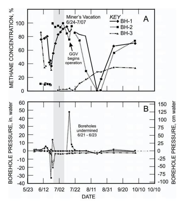
Figure 34.—Methane concentration (A) and static shut-in pressures (B) measured in the boreholes during progress of mining.
