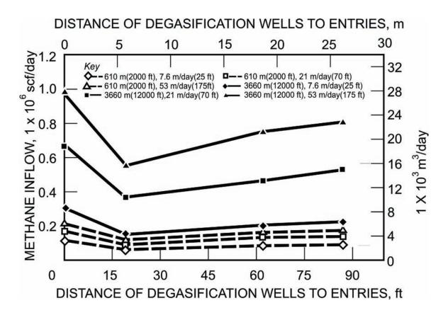
Figure 3.—Effect of mining rate and shielding well proximity when mining 610-m and 3,660-m (2,000-ft and 12,000-ft) long entries.
