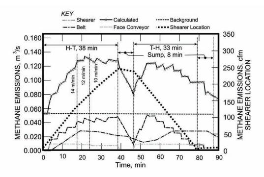
Figure 21.—Calculated influence of variable shearer transit speed pass for a 488-m (1,600-ft) longwall face.
