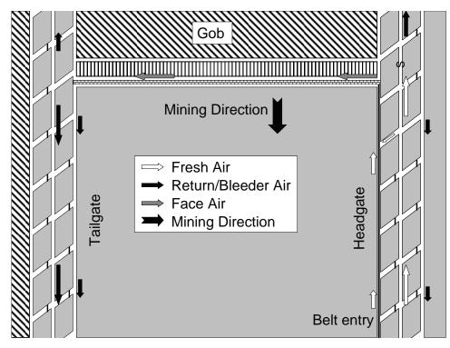
Figure 15.—Ventilation configuration at the study site (not to scale).
