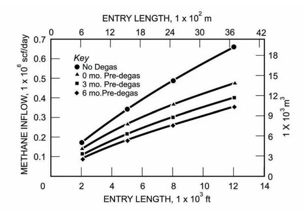
Figure 2.—Methane inflow rate predictions for different development lengths and various premining degasification durations.
