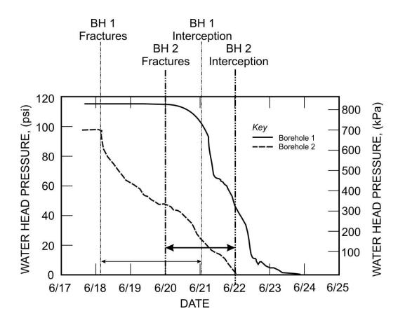
Figure 31.—Water head change as a function of time in boreholes monitoring Sewickley (BH–1) and shale-limestone (BH–2) intervals.
