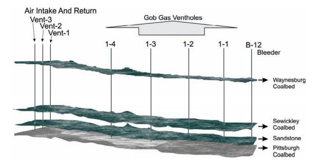
Figure 26.—Study mine for wider longwall faces: grid model of a new mining district in the Pittsburgh Coalbed.
