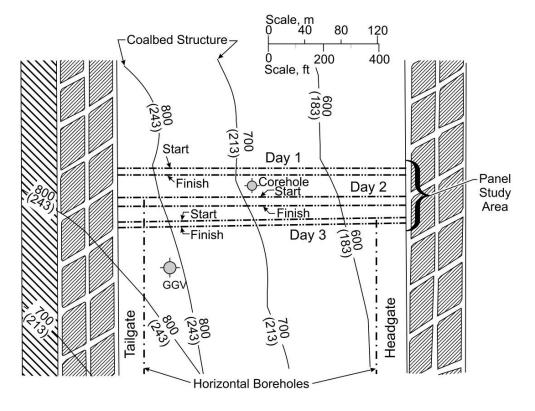
Figure 16.—Actual portions of the study panel monitored for face methane emissions and associated methane drainage borehole locations.
