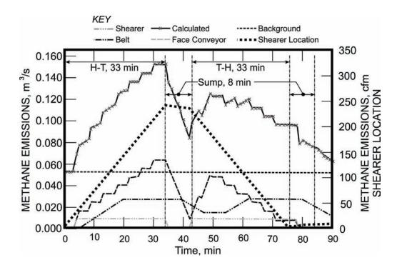
Figure 20.—Calculated methane emissions for two full cuts without delays for a 488-m (1,600-ft) longwall face.
