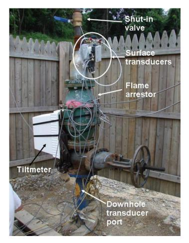
Figure 30.—Wellhead arrangement for monitoring boreholes.
