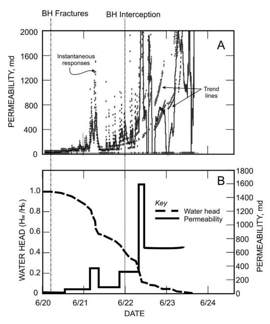
Figure 33.—A: BH–2 instantaneous change in the permeabilities of monitored horizons during mining; B: BH–2 average permeabilities. ( $H_w$  = height of water;  $H_o$  = initial height of water.)
