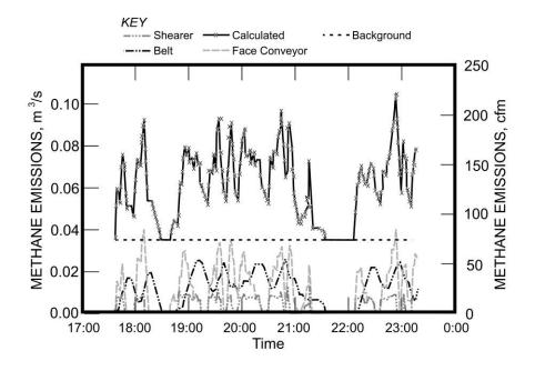
Figure 19.—Calculated individual methane contributors and total calculated methane emissions for study day 1.
