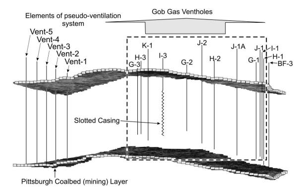
Figure 22.—Three-dimensional representation of grid model of the study area that shows the Waynesburg *(top layer)* and Pittsburgh *(bottom layer)* Coalbeds. Also shown are GGVs, their placement, completion representation, and elements of a pseudo-ventilation system.
