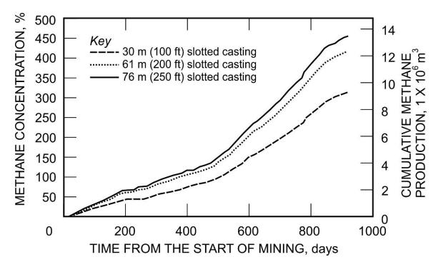
Figure 23.—Simulated cumulative methane production from ventholes with varying lengths of slotted casing.
