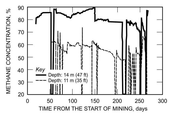
Figure 25.—Actual methane concentrations measured in the gas production stream from two GGVs completed to different depths above the Pittsburgh Coalbed on the same longwall panel.
