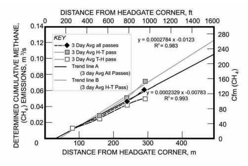
Figure 18.—Methane emission prediction curves for the Pittsburgh Coalbed.
