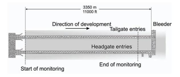
Figure 1.—The modeled longwall panel showing entry sections where mining and ventilation data were gathered during development mining.
