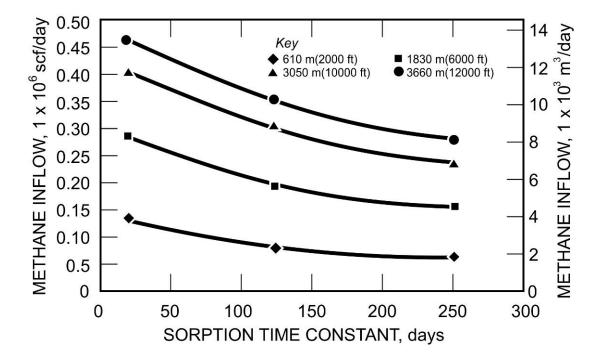
Figure 7.—Influence of sorption time constant of the coal on reservoir-simulated methane inflow rates during mining.
