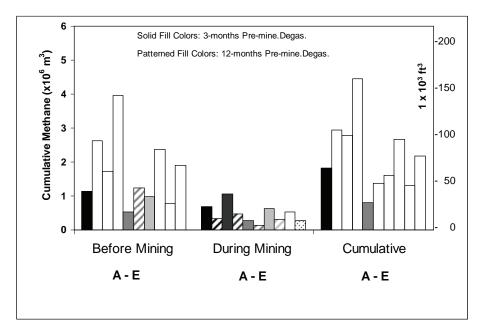
Figure 11.—Performances of different horizontal methane drainage borehole patterns shown in Figure 9 during different phases of degasification, after 3 and 12 months of premining degasification.
