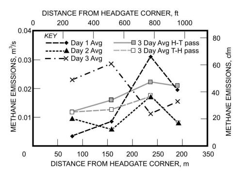
Figure 17.—Average methane emission rates for each day of study determined for each face segment.
