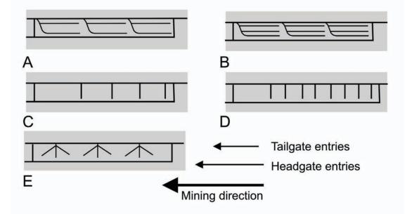
Figure 9.—Horizontal methane drainage borehole patterns modeled for degasification of the longwall panel *(not to scale)*.
