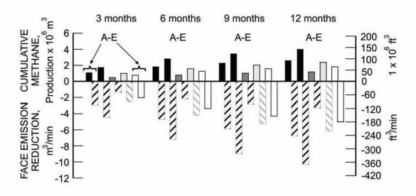
Figure 10.—Cumulative methane production and possible reductions in longwall face emission rates for different premining methane drainage time intervals and different horizontal borehole patterns (A through E).
