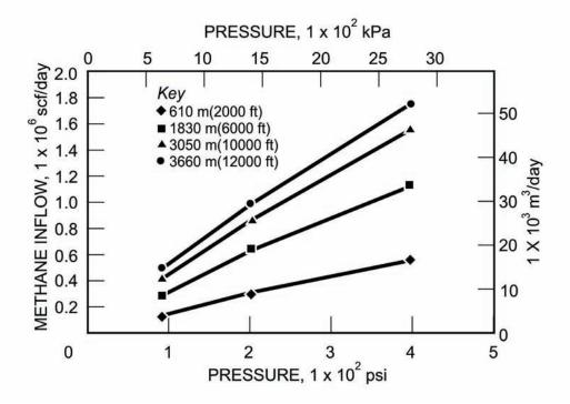
Figure 5.—Effects of coalbed pressure on predicted methane inflow rates into development entries using reservoir simulations.
