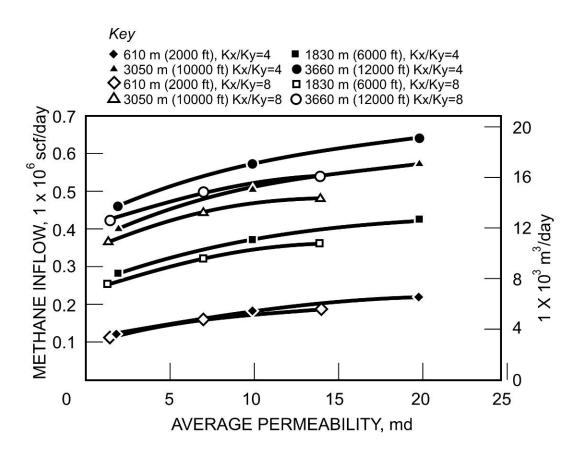
Figure 4.—Reservoir model predictions of methane inflow rate changes with permeability, permeability anisotropy, and entry length.
