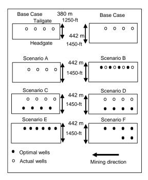
Figure 27.—Schematic representation of GGV configurations for the simulation of methane control options on wider longwall panels.
