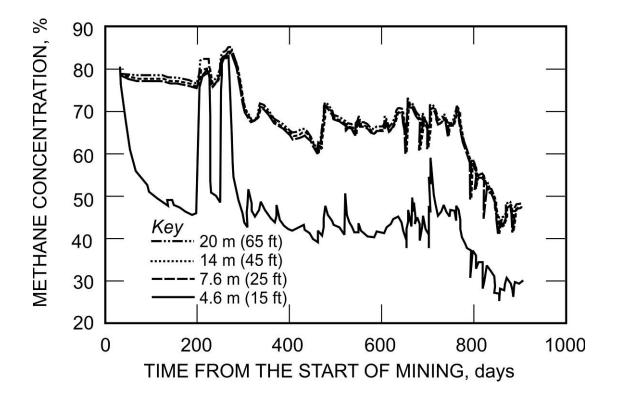
Figure 24.—Simulated methane concentrations in the gas production stream from ventholes completed to varying depths above the Pittsburgh Coalbed.
