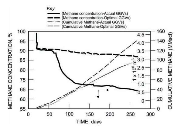
Figure 28.—Comparison of the performance of actual GGVs at the study site with the optimal GGVs for the 442-m (1,450-ft) wide panel.
