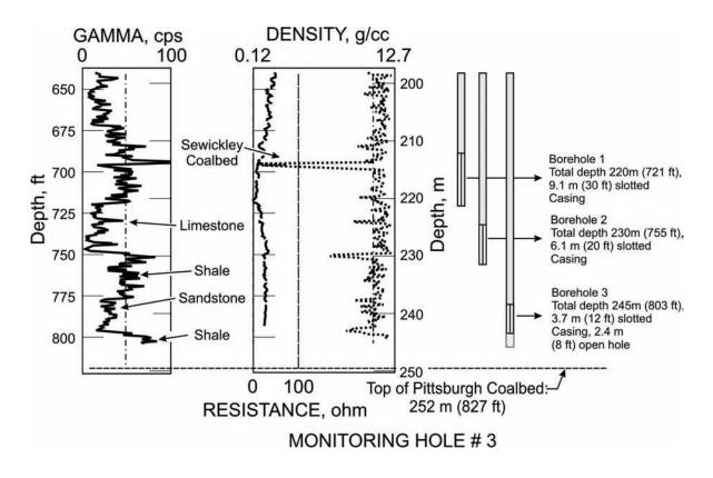
Figure 29.—Stratigraphy and downhole configurations for NIOSH BME. (TD = total depth.)
