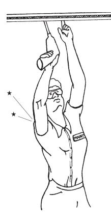
Good ergonomics can eliminate some of the awkward tasks associated with maintenance and repair. Moreover, these same considerations can reduce down time for repairs, improve inspection of critical components and reduce failure-related accidents.
