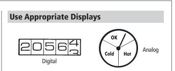
Often, the type of display used will help provide the user with the easiest and most accurate way to gain necessary information. Digital displays are usually best when precise information is needed. However, analog gauges tend to be faster and clearer for general indication.
