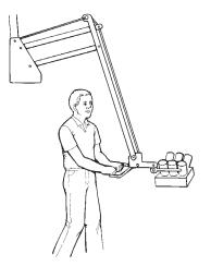
**Use power tools, machines and cylinders** — Perhaps the most obvious way to reduce force is to completely mechanize the activity. Air and hydraulic cylinders are particularly useful when moderate force is needed.
