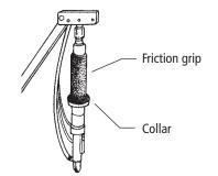
**Increase contact friction or use a collar** — If a grip is slippery, you must squeeze harder to accomplish the same task. One common improvement is to cover the grip with a material that provides higher friction. In cases where the force applied is coaxial to the grip, providing a collar or stop on the grip can reduce grasping force.
