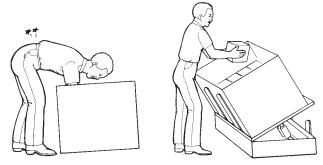
The "inverted V-curve" is a serious injury-producing posture; it can be avoided with use of a tilter. Twisting motions, especially with a heavy load, can also cause injury.
