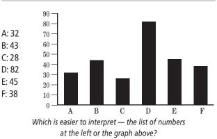
Humans are good at recognizing patterns quickly and accurately. That's why graphs are much easier to read and interpret than columns of numbers. Bar graphs are especially good for comparing numbers, and line graphs are good for showing trends. A final general area of ergonomics has to do with the underlying design of work and related issues:
