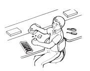
**Make cutouts** — An increasingly common approach is to make a cutout in the work surface. Cutouts reduce reaches yet still allow large workspaces.
