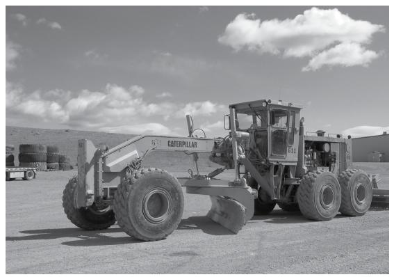
Figure A.13. Caterpillar 16G motor grader.
