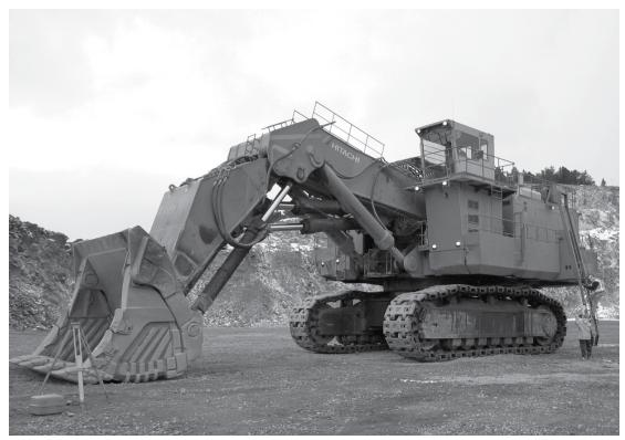
Figure A.7. Hitachi EX5500 excavator.
