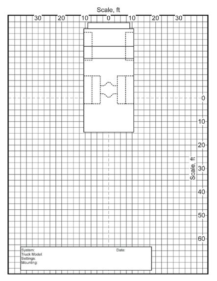
Figure B.1. Example of test grid for rear detection zone.
