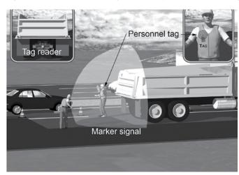
Figure 3. Illustration of tag-based system operation.
