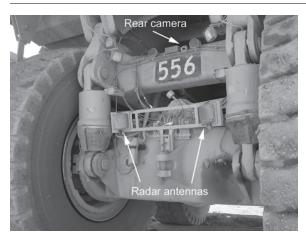
**Figure 5**. Preco radar antennas and Vision Techniques camera mounted on the rear of a haul truck.
