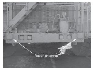
Figure 6. Preco radar antennas mounted on the front bumper of a haul truck.
