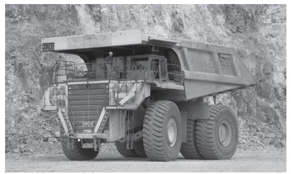
Figure A.1. Euclid EH4500 280-ton-capacity haul truck.
