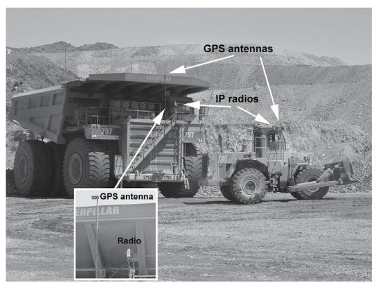
Figure 22. Tests of a GPS-based proximity warning system.
