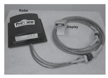
**Figure 1.** An example of a radar-based proximity warning system (early version of the Preview radar system by Preco Electronics).
