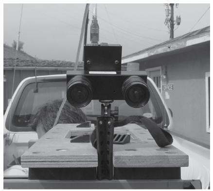
Figure 23. Stereo camera system.
