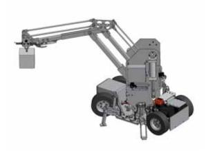
Figure 2.—Manipulator shown loaded with stabilizers activated.
