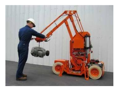
Figure 1.—Manipulator in operation.
