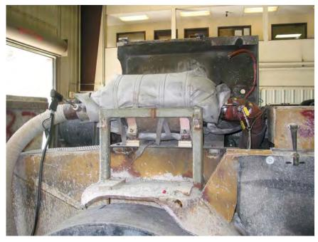
Figure 2.—CleanAIR Systems DPF system on truck #92133.
