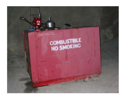
Figure 8.—Fueling station in isolated zone.
