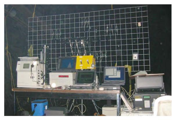
Figure 13.—Downstream sampling station showing instrumentation and grid supporting DPM samplers, anemometer, and iTX gas monitor.
