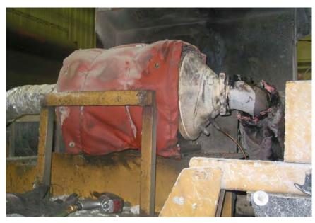
Figure 1.—Engelhard DPX DPF system on truck #92128.
