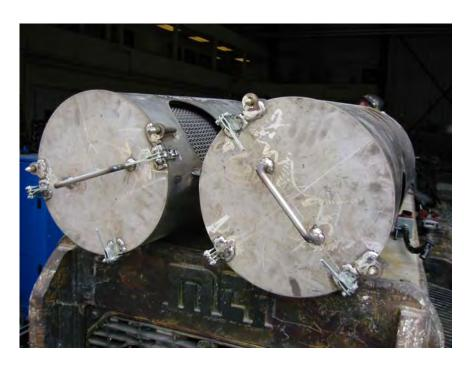
Figure 4.—Mac's Mining Repair filtration system on LHD #92506 used for testing Donaldson P604516 and Filter Services DFEs.
