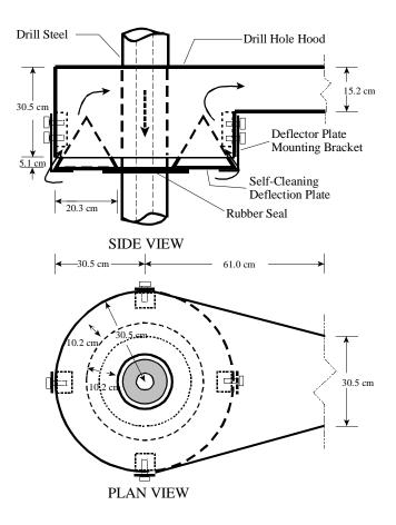
Figure 1.Cinlet hood design tested in laboratory.
