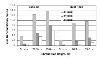
Figure 2.CDust escaping the laboratory drill shroud.
