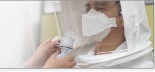
A worker undergoing qualitative fit testing
