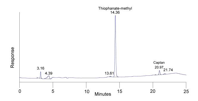
**Figure 1** This chromatogram shows results from a spiked patch sample that was extracted and analyzed by this method. The analyte quantities were: thiophanate-methyl -  $200 \mu g$ /sample and captan-  $50 \mu g$ /sample.
