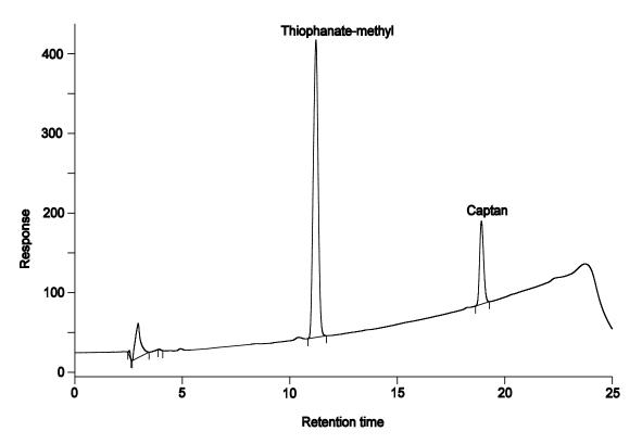
**Figure 1**. A typical chromatogram from the analysis of a hand rinse storage sample. The concentrations of the analytes shown here are: thiophanate-methyl -  $226 \ \mu g/mL$  and captan -  $175 \ \mu g/mL$ .
