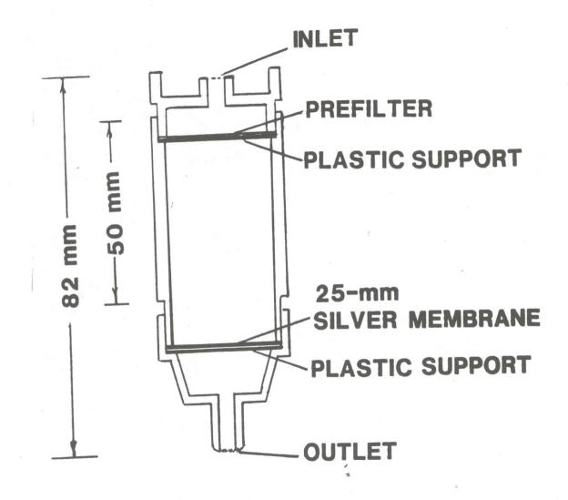
Figure 1. Silver Filter Sampler
