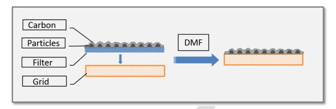
**Fig.3.** Removal of residual MCE polymer from carbon-coated sample by dimethylformamide (DMF). After polymer removal, only particles embedded in the carbon film remain on the grid.
