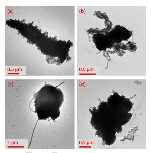
Fig. 6. Examples of CNT matrix particles: (a)-(d) collected from workplaces.
