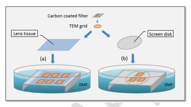
**Fig. 2.** Sample transfer and final processing: place a piece of lens tissue (a) or a stainless steel screen disk (b) on a stainless screen platform in a Jaffe wick washer filled with dimethylformamide (DMF). Sides of the platform are bent to keep sample grids above the solvent level. Depending on size, multiple disks can be used to hold grids.
