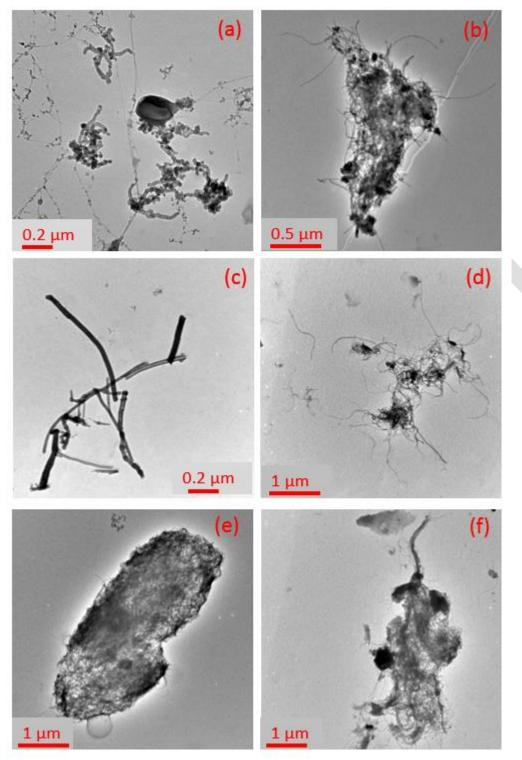
**Fig. 5.** Examples of CNT/CNF clusters: (a)-(f) collected from workplaces.
