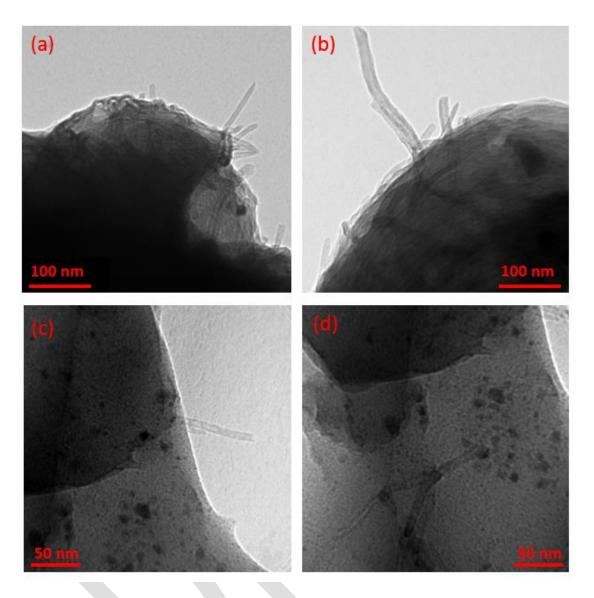
Fig. 9. Examples of CNT particles embedded in polymer composite: (a)-(d).
