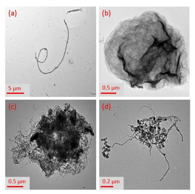
**Fig. 8.** CNT particles in personal breathing zone samples collected from various sites: (a) MWCNT fiber (polymer composite site), b) SWCNT agglomerate from aerosolized, aqueous suspension (electronics site), c) MWCNT agglomerate (composites/thermoplastics site), and d) MWCNT agglomerate (primary manufacturer of CNT).
