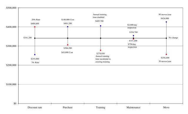
Figure 2. Summary of sensitivity analysis completed on refuge chamber costs.
