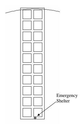
Figure A1. Area available for mining for 3 entry system: Arc is limit for 1000 ft distance away from face assuming linear advance.
