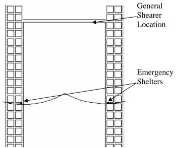
Figure A3. Area available for mining for longwall system: Arcs are limits for 1000 ft distance away from face assuming linear advance.
