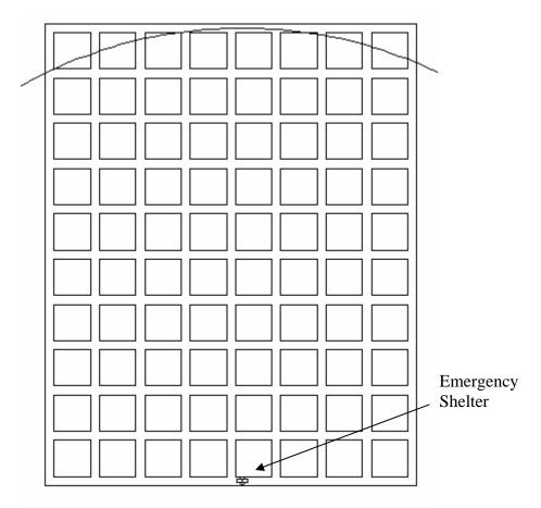
Figure A2. Area available for mining for 9 entry system: Arc is limit for 1000 ft distance away from face assuming linear advance.
