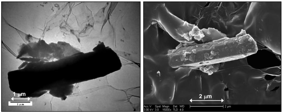
What appears to be a long, thin particle in the TEM image is revealed in the FESEM image to be a prismatic particle coming out of the plane of the projection screen; the particle is clearly not a fiber.
