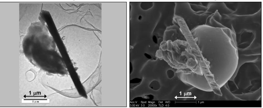
What appears to be a long, thin fiber in the TEM image is revealed in the FESEM image to be a prismatic particle coming out of the plane of the projection screen; the particle is clearly not asbestiform.
