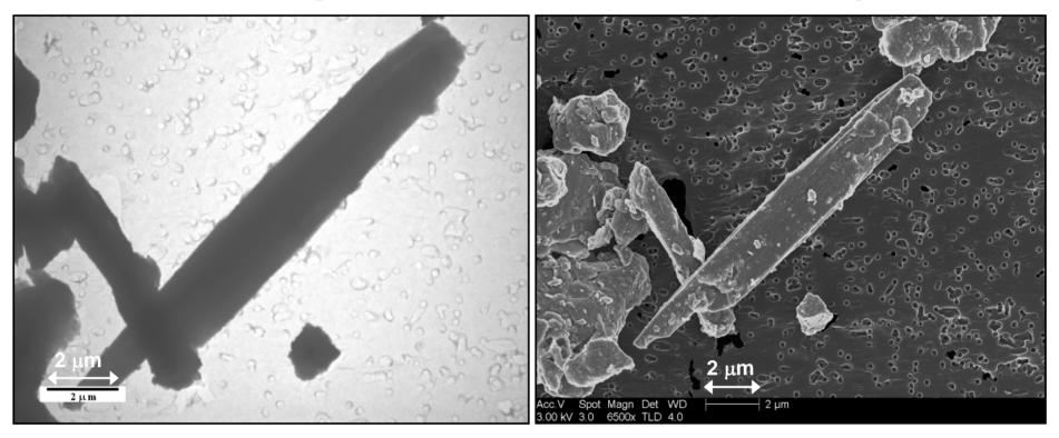
> What appears to be a long, thin fiber in the TEM image is revealed in the FESEM image to be a prismatic particle; the particle is clearly not asbestiform. RIG
