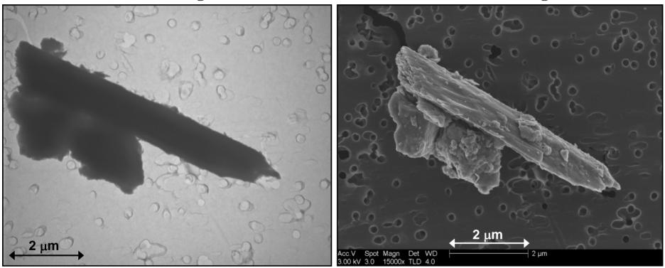
What appears to be a long, thin particle in the TEM image is revealed in the FESEM image to be a prismatic particle; the particle is clearly not a fiber.
