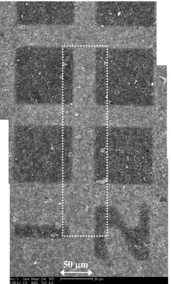
Long, thin fiber traverses ~2.5 grid squares, traveling along the grid bar so that it is not visible in the TEM
