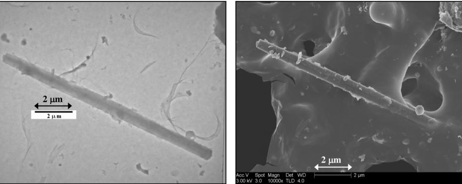
What appears to be a long, thin fiber in the TEM image is revealed in the FESEM image to be a particle coming out of the plane of the projection screen; the particle is clearly not asbestiform.
