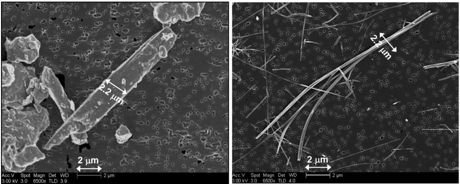
The concept that a significant portion of cleavage fragments have the same diameter as airborne asbestos fibers is a myth.
