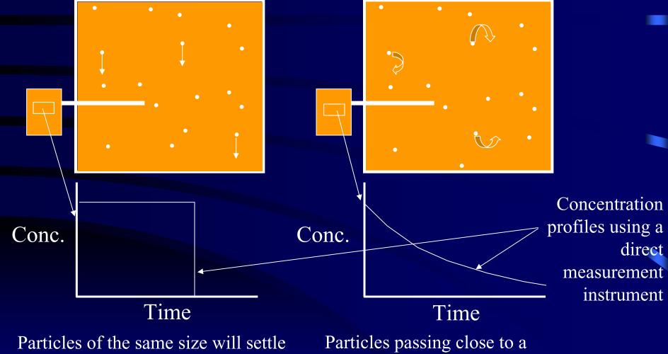
at the same speed in still or stagnant air Particles passing close to a horizontal surface can settle, but the rest will continue to be stirred.
