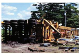
Figure 6. Mobile tower crane tip-over attempting to hoist water tank. (Photo courtesy of Iowa FACE Program)
