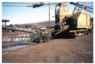
Figure 7. Boom collapse during crane disassembly.
