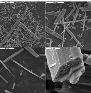
Figure 1. Massive tremolite (var. hexagonite) ground with a pestle in a mortar to produce cleavage fragments. Unground sample (upper left) and scanning electron micrographs at various magnifications are shown. Photograph courtesy of USGS.
