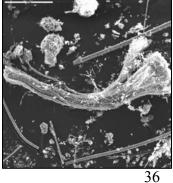
Figure 8. SEM image of a chrysotile bundle (center) and glass fibers from World Trade Center dust sample. Photograph courtesy of USGS
