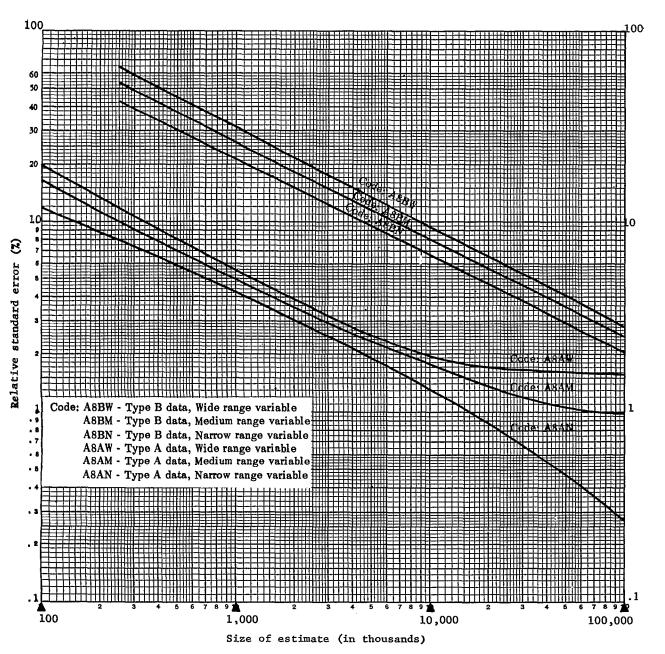
Example of use of chart: An aggregate of 5,000,000 (on scale at bottom of chart) for a Narrow range type A statistic (code: A8AN) has a relative standard error of 1.9 percent, read from scale at left side of chart, or a standard error of 95,000 (1.9 percent of 5,000,000). For a Wide range type B statistic (code: A8BW), an aggregate of 10,000,000 has a relative error of 9.3 percent or a standard error of 930,000 (9.3 percent of 10,000,000).
