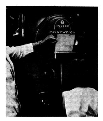
Figure 9. Automatic recording of scale readings.
