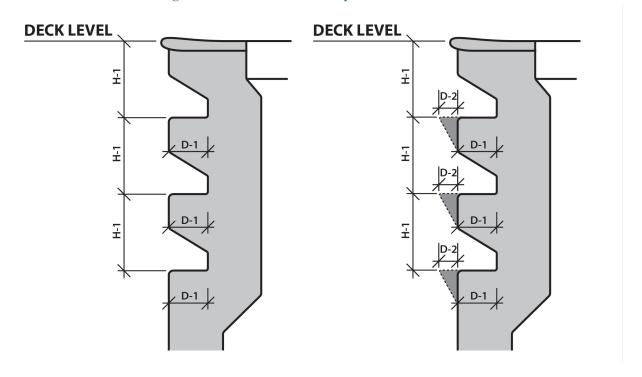
Figure 4.5.7.4.2: Recessed Step Dimensions: Front View
